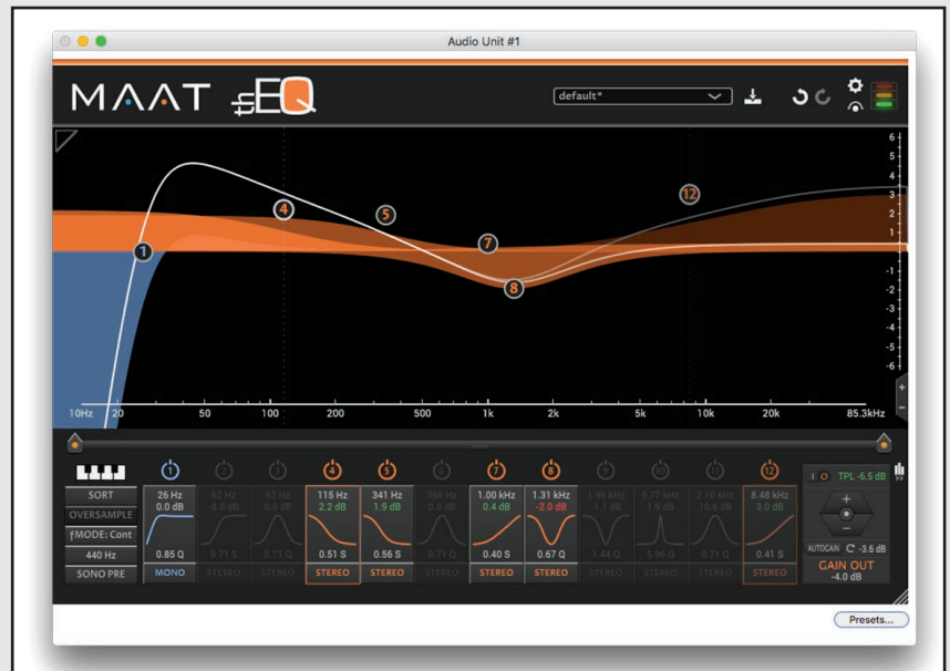
Photo 1: This EQ combines an upward low-frequency tilt with a midband scoop and a steep low-frequency roll-off to limit excursion. Band #12 provides a 3 dB lift at higher frequencies to correct for the dark aspect I mentioned.
