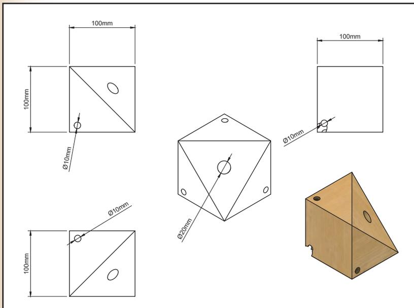
Figure 4: Here is the microphone block assembly.
