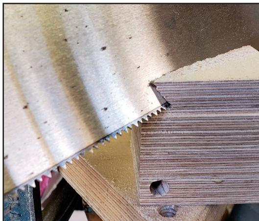
length and from the 18 mm sheet cut five squares each 90 mm on the side. Use these five layers of plywood to produce a cube. Drill the three holes for the dowels on the sides of the cube. This is then cut on the diagonal into two parts (see **Figure 4** and **Photo 2**).
