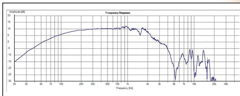
Figure 5: This is the external very-near-field response.
