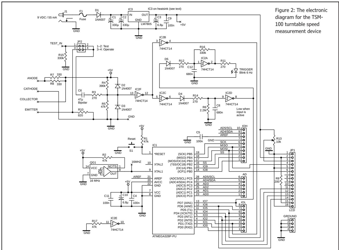
Figure 2: The electronic diagram for the TSM-100 turntable speed measurement device
