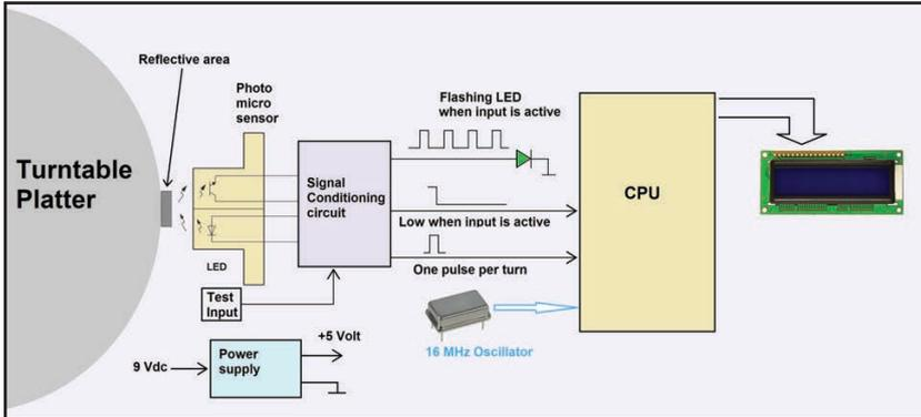
Figure 1: The block diagram of the device
