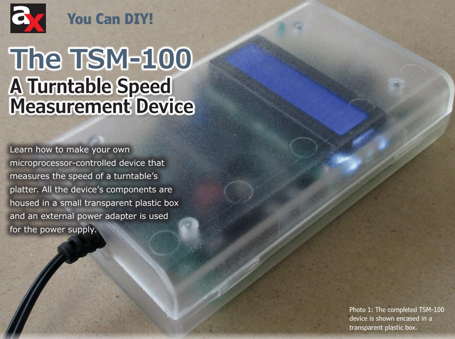
Photo 1: The completed TSM-100 device is shown encased in a transparent plastic box.
