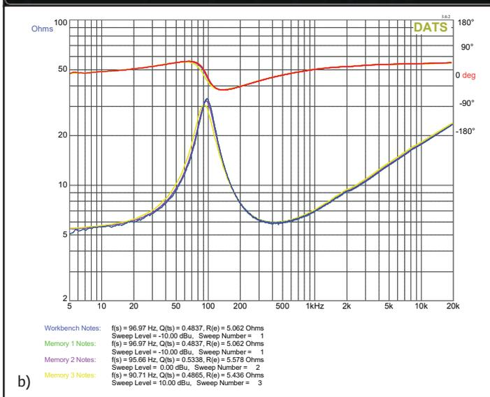
Figure 6: The set-up panel for Linearity testing provides settings for signal level, number of sweeps, and the decibel change per sweep (a). Linearity test results are plotted for three sweeps in 10 dB steps up to the maximum amplitude of +10 dBu for the Peerless 850102 (b).
