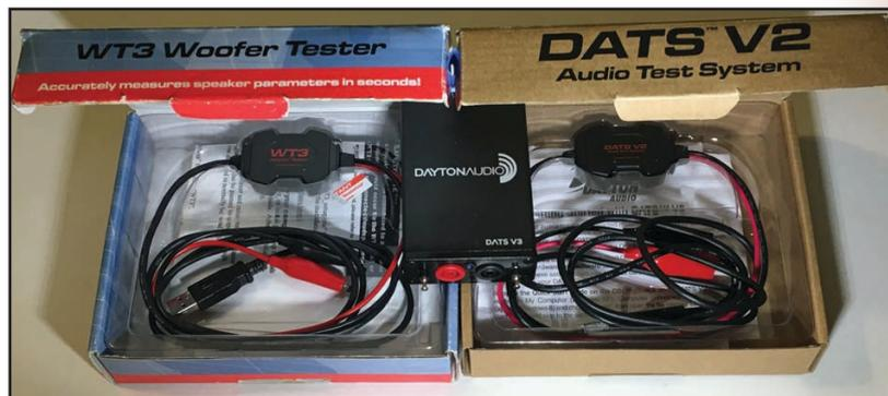
Photo 3: Three generations of DATS are shown, including the WT3 (left), the DATS V2 (right), and the DATS V3 (center).
