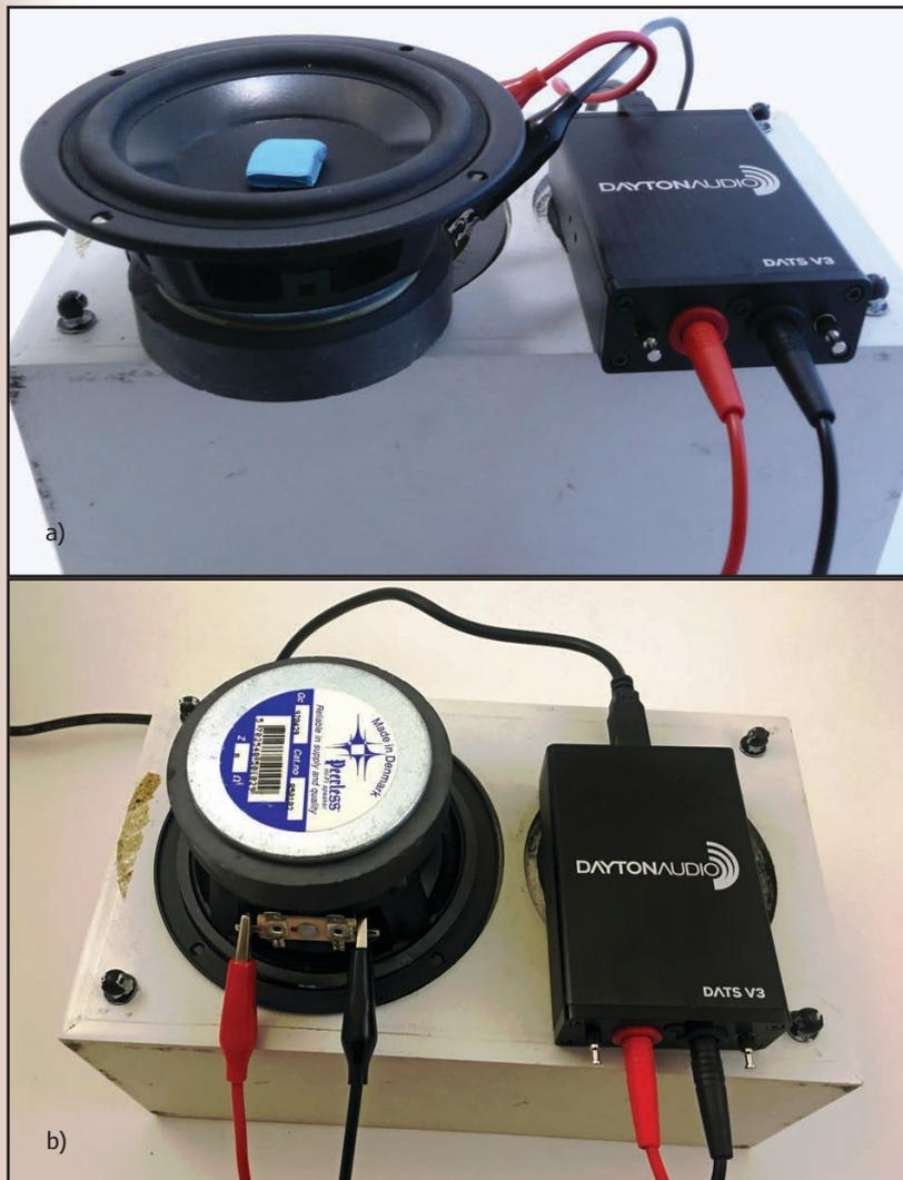
Photo 4: The DUT is tested using the Vas Added Mass method (a) and the DUT is tested using the Vas Test Box method (b).
