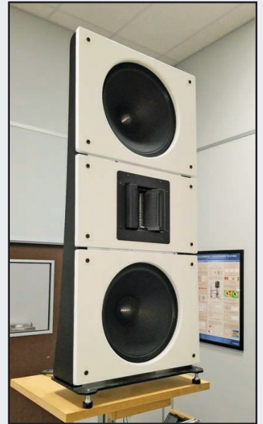
Photo 1: PureAudioProject's Trio15, featuring the ESS Heil AMT 1, was measured at Warkwyn's facility using the Klippel Near-Field Scanning system (NFS).
