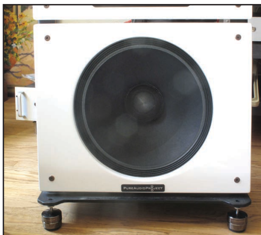
Photo 2: An Eminence direct radiator in situ
