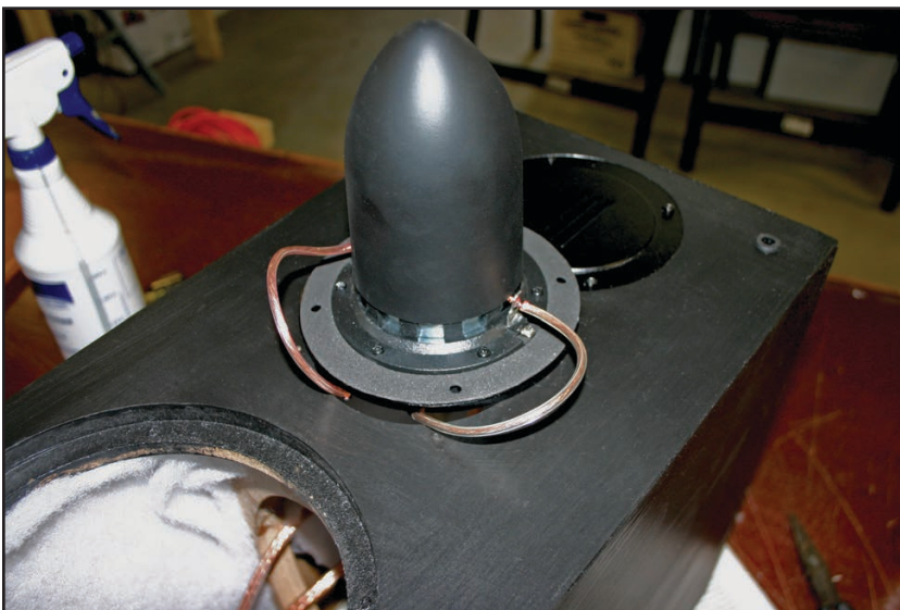
Photo 9: I wired the speakers using the supplied cable. The polyester battens lining the insides can be seen.
