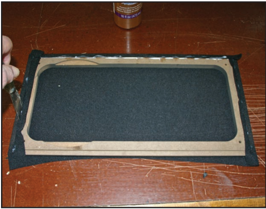
Photo 7: I applied the grill cloth into the pre-milled grills using a thin putty knife to stuff the cloth into the glue-filled grooves.
