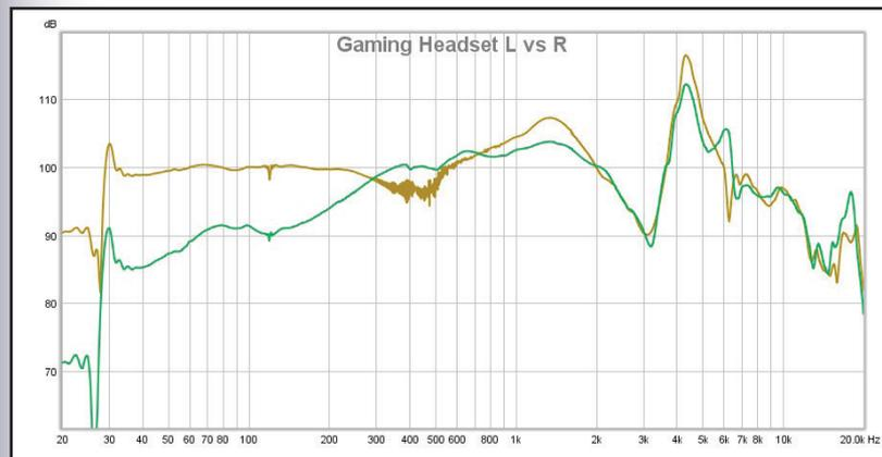
Figure 8: Using the EARS to test some gaming headphones that sounded bad immediately showed the problems.
