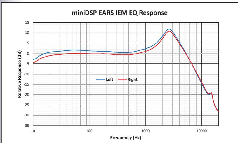
Figure 3: miniDSP also provides IEM equalization curves for users of in-ear headphones where the HRTF contribution of the pinnae are minimized.
