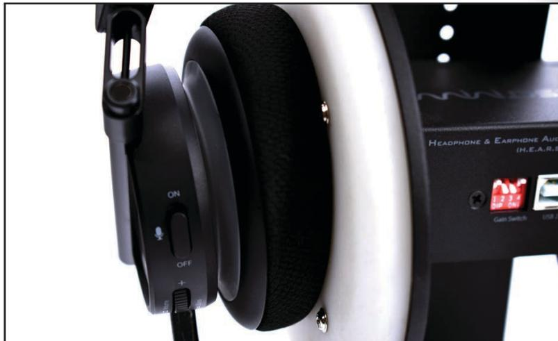
Photo 2: The screws used to fasten the rubber pinnae to the test fixture can compromise the seal of circumaural headphones. These should be changed to countersunk screws. (Photo courtesy of Cynthia Wenslow)
