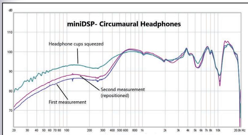
Figure 6: The measured bass response is greatly affected by headphone positioning and tension. Blue curve = first measurement. Magenta curve = measurement after repositioning the headphones. Green curve = measurement with pressure applied to the headphone cups.
