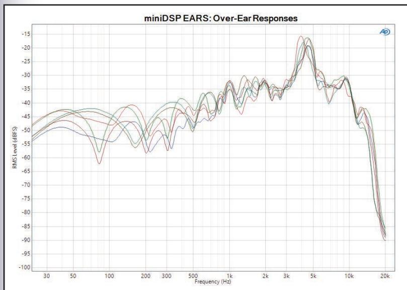
Figure 5: The variation in frequency response caused by removing and replacing the headsets between repeated measurements demonstrates the need to average over multiple repetitions.
