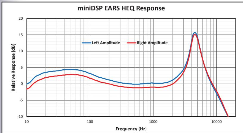
Figure 2: The HEQ equalization curves account for the acoustic effects of the simulated pinnae and ear canal, and are a starting point for users to equalize to a flat frequency response.
