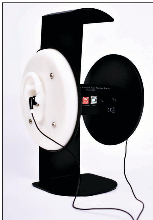
Photo 1: The miniDSP EARS headphone jig is a basic and inexpensive alternative to laboratory-grade measurement systems. (Photo courtesy of Cynthia Wenslow)
