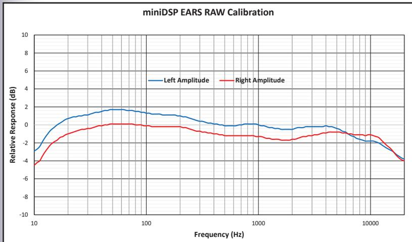
Figure 1: The RAW EQ files provided with the miniDSP EARS compensate for the frequency response of the embedded electret microphone capsules.
