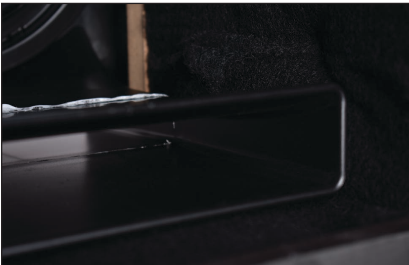
Photo 4: The oddly shaped port is made from an injection-molded plastic and is flared to reduce turbulence.
