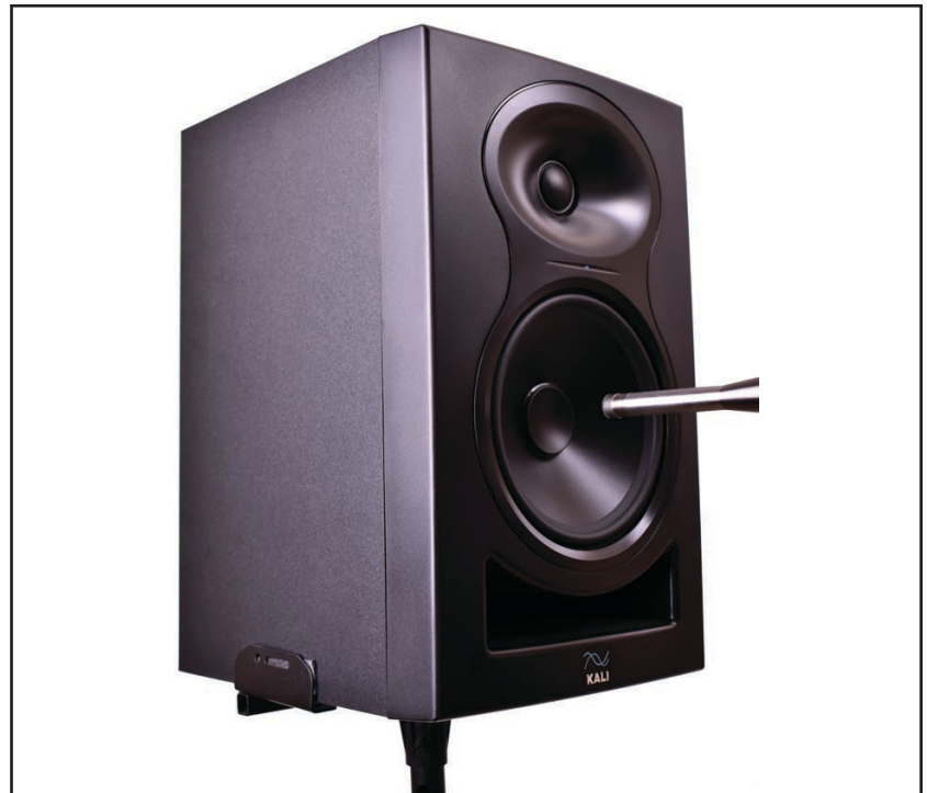
Photo 5: Near-field measurement of the Kali Audio LP-6 Studio Monitor shows excellent bass extension and quality.
