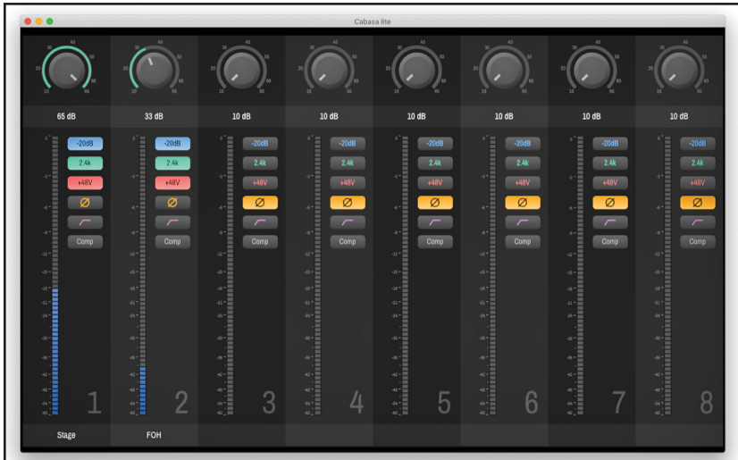
Photo 5: A third-party web browser UI controls all the AES70 objects in a Focusrite MP8R (an eight-channel remote-controlled mic preamp and A-D interface for Dante AoIP networks). It would be possible to unify each strip with additional parameters (e.g., a console channel) and utilize both over Dante/AES67 + AES70.
