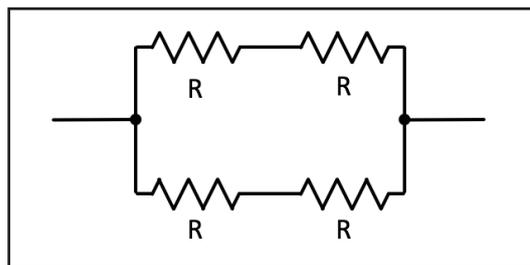
Figure 3: Any resistor of value R may also be constructed from multiple elements to further reduce heating.
