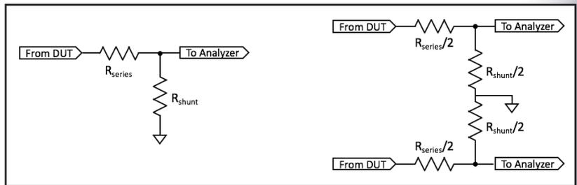
Figure 1: The U-pad is simply two identical L-pads placed back-to-back in a mirrored configuration—each side attenuating one side of the balanced signal.
