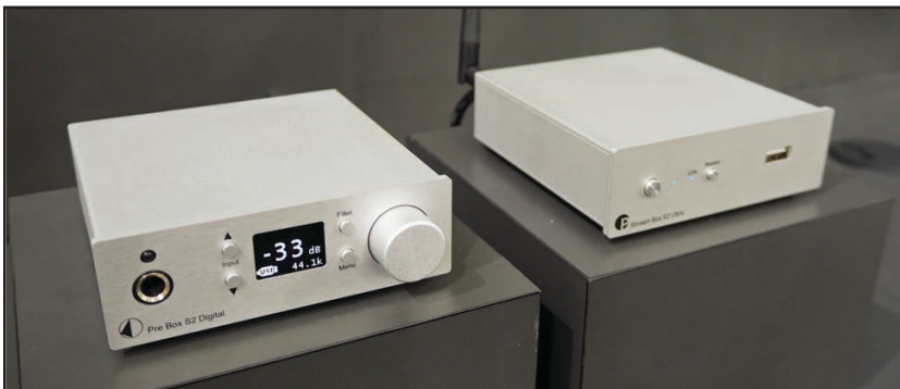
These tiny things are the Pre Box S2 Digital DAC, using ESS Sabre converters and supporting up to 32-bit/768 kHz PCM and DSD512, as well as hardware MQA unfolding ($349); and the Stream Box S2 Ultra ($799) a Roon-ready Wi-Fi or Ethernet music streamer.
