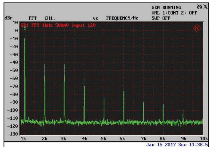
Figure 7: At this operating point, a Fast Fourier Transform (FFT) shows that the second and third harmonic distortion products were nearly equal in level at -40 dB, with dropping levels for higher order products.
