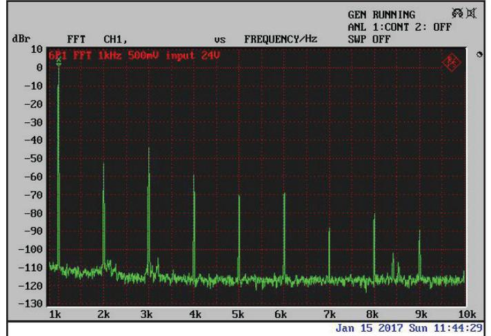
Figure 9: The FFT at 24 V shows that the second harmonic product has dropped, and now the third is the highest, at about -43 dB.
