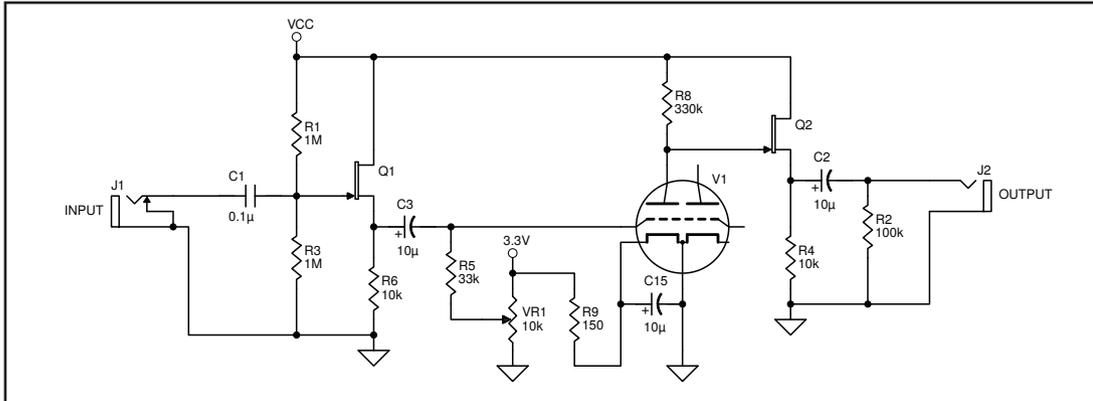
Figure 4: The Korg application circuit uses simple JFET source followers to buffer the signal in and out of the Nutube.
