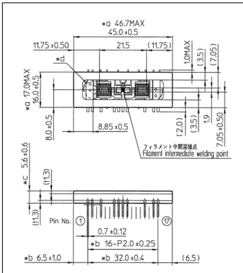
Figure 3: The package measures 45 mm x 16 mm and is designed to mount to a PCB, with pins spaced on 2 mm centers.
