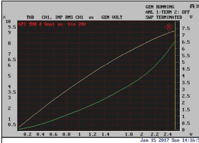
Figure 8: Using the same operating point and load, things improve considerably at a higher supply voltage. Here is the same circuit running from 24 V.
