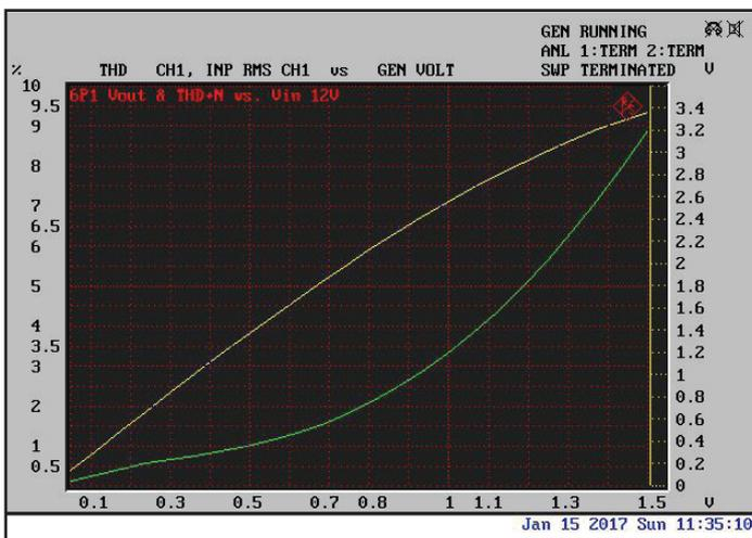
Figure 6: With 12 V gain and distortion, the THD increases with the level.
