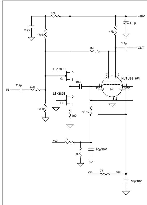
Figure 10: I set the MP7770 Class-D circuit up for slightly lower gain than it would normally have and used the Nutube 6P1 as an input stage, feeding a JFET phase splitter.
