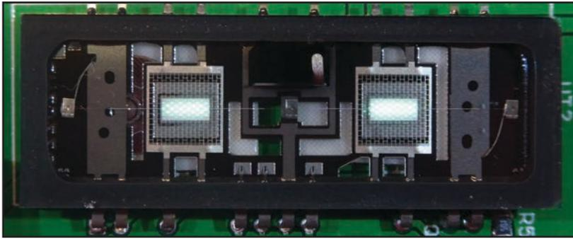
Photo 2: The Nutube resembles an old 40-pin DIP IC package, but only has pins along one edge.
