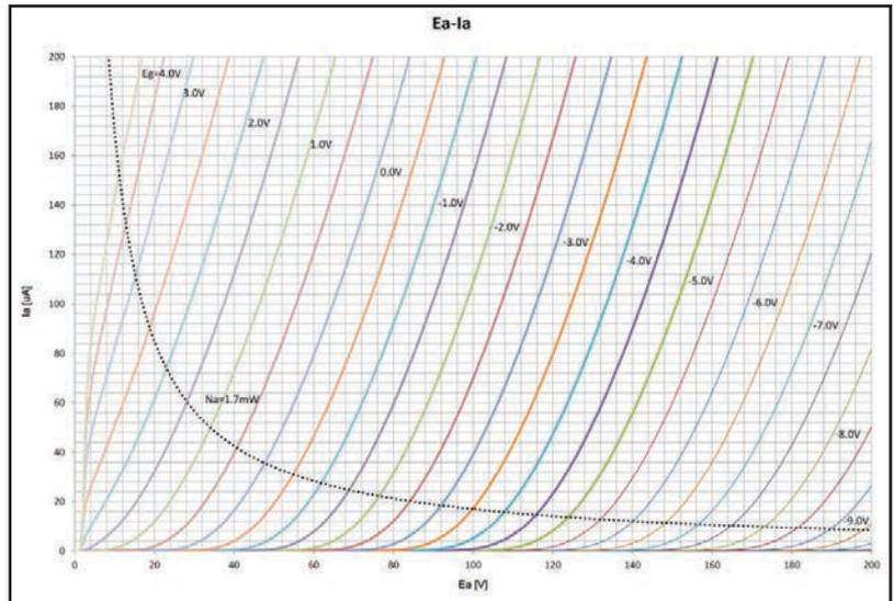
Figure 1: The curves are typical for a triode and quite linear.
