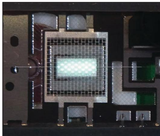
Photo 1: The 6P1 triode has a fine coated wire running across the device.
