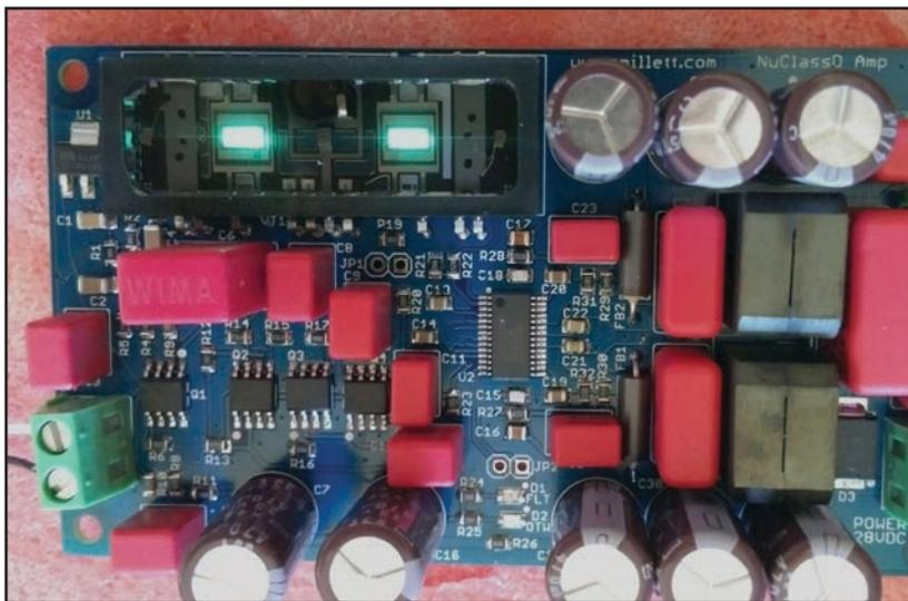
Photo 3: As an experiment, I designed and built a hybrid amplifier using the Nutube 6P1 in conjunction with a self-oscillating Class-D amplifier IC, the MP7770 from Monolithic Power Systems.
