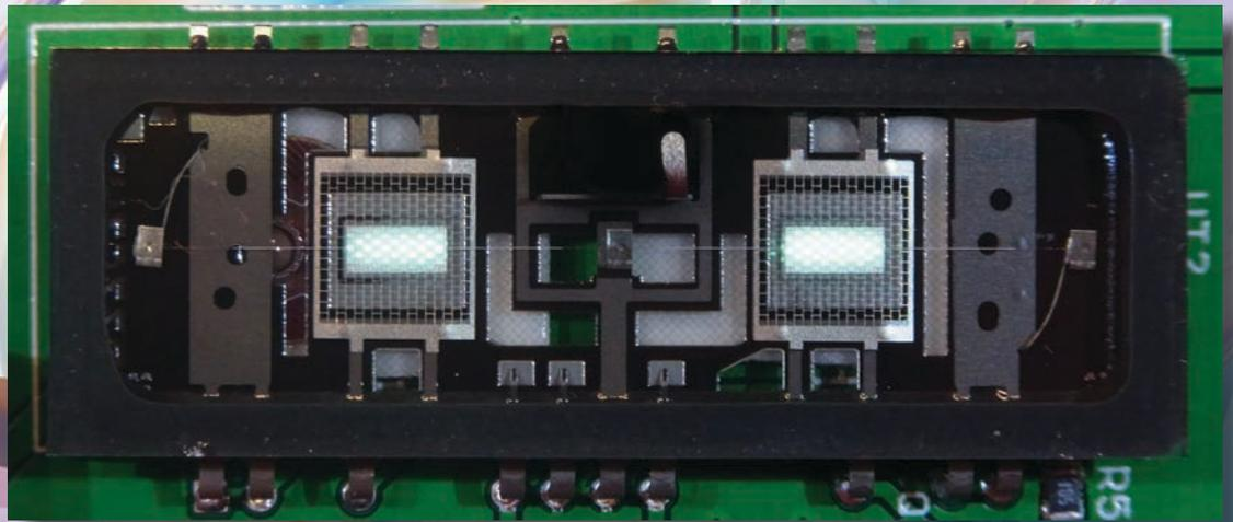
Learn more about the Korg Nutube 6P1—a new miniature, low-power dual directly heated triode device developed by Korg (of musical instrument fame) and Noritake Itron, a Japanese manufacturer of vacuum fluorescent displays. Although it is a true directly heated triode, it is manufactured differently than traditional vacuum tubes, which gives it some unique attributes.
