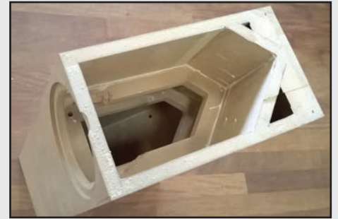
Looking into the lower portion of the Rinjani prototype cabinet. This photo also reveals internal bracing and the inner wedge-shaped rear wall, behind the midwoofers only, that significantly reduces the reflected sound wave.
