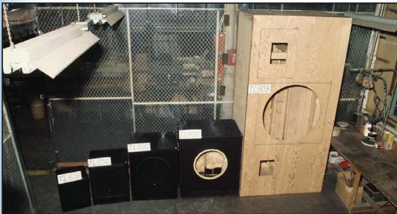
Photo 5: The complete line of single-driver direct-radiator TL bass boxes are shown from left to right: the TL806, the TL606, the TL505, the TL405, and the TL303. These boxes housed respectively, from left to right: the EVM12L, the EVM15L, the EVM18B (two boxes) and the EV 30W 30" driver.
