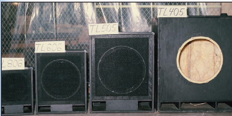
Photo 6: This is a close up view of the four single-driver TL bass boxes. Note ports on the bottom of the boxes. The left three boxes are set up for the step-down mode of operation with the center port closed. The right box is set up for normal operation with all three ports open.
