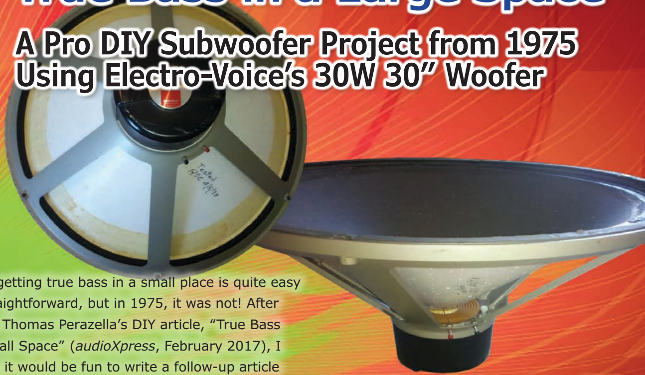
Photo 1: Bottom and side images of the Electro-Voice 30W woofer (Photos courtesy of Canuck Audio Mart)
