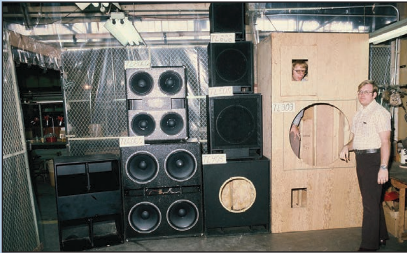
Photo 4: The complete line of TL bass boxes including seven direct radiators and two folded-horn boxes. The larger folded-horn box (TL4050) is not shown. The 1975 photo shows Glen Meyer inside the TL303 box and Larry Driskill standing in front.
