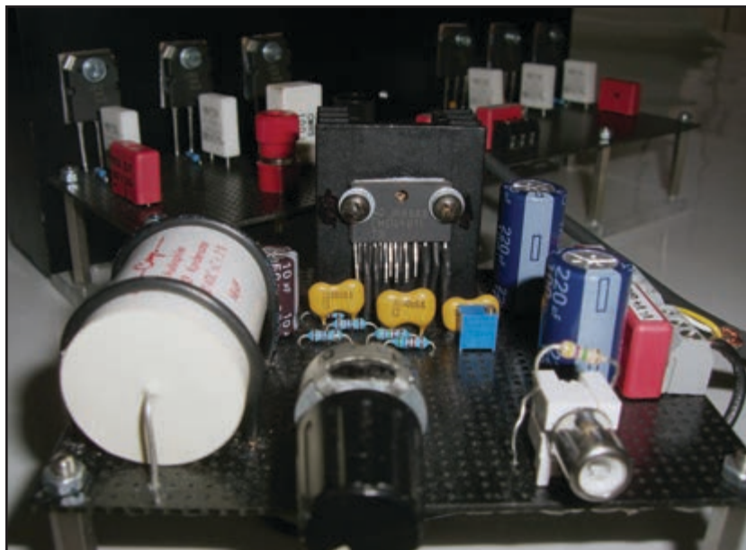
Photo 5: The LME49811 stage is shown in the front with the power stage at the back.
