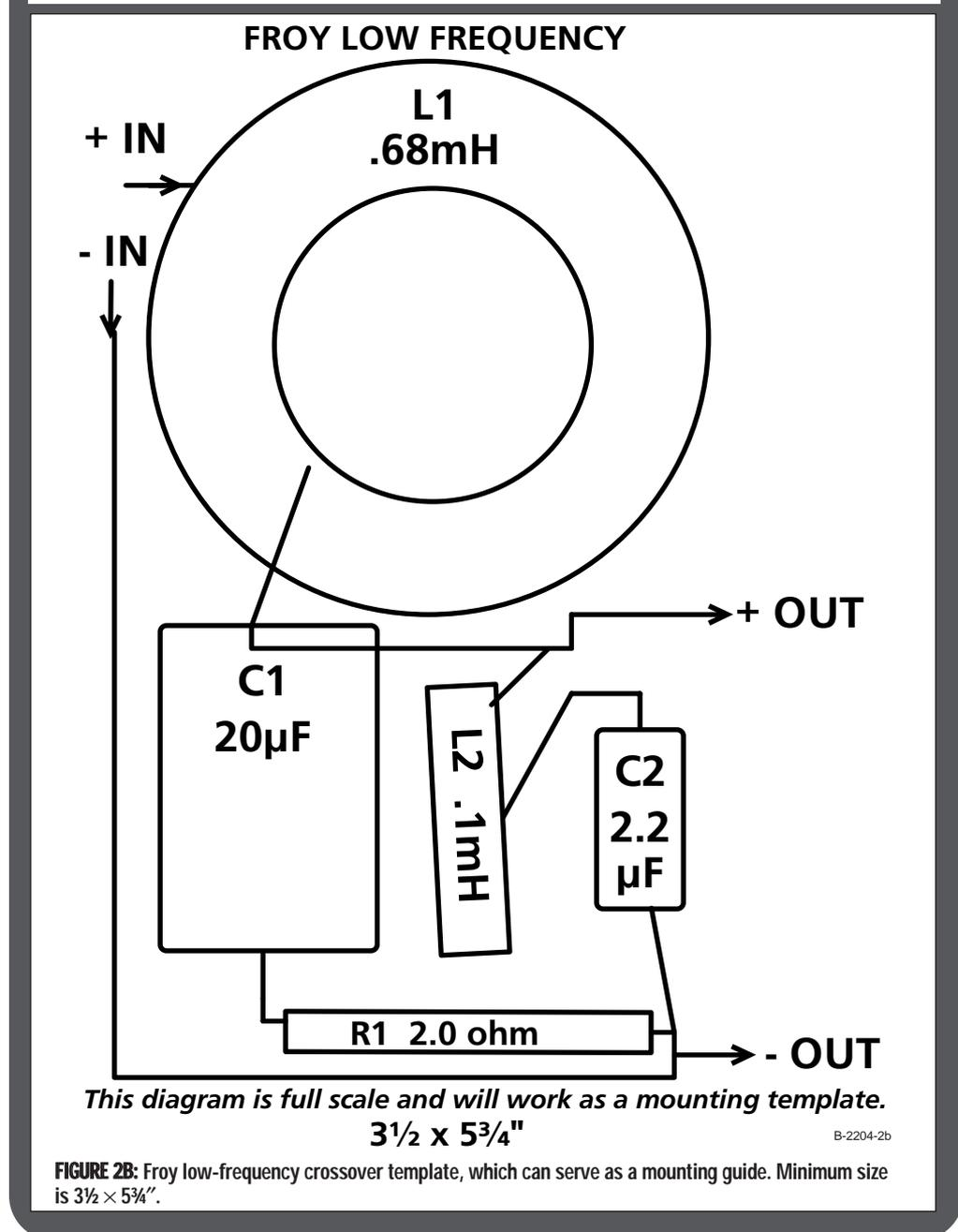
**This diagram is full scale and will work as a mounting template. 3 1/2 x 5 3/4"**
