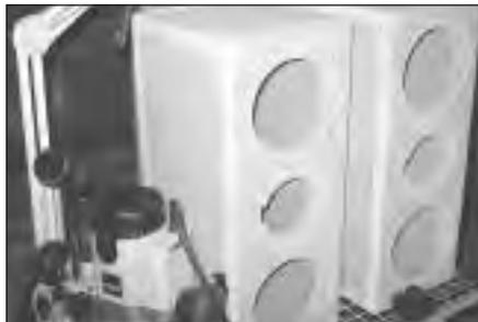
**PHOTO 7:** All box edges were rounded with a router, 5/8" bit. The router is a new style DeWalt equipped with a dust port for connection to a vacuum.
