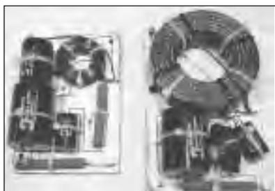
**PHOTO 8:** The two assembled crossover networks, HF on the left, LF on the right. Components are held in place with cable ties. Stud terminals are press-fit into the 1/8" Masonite.
