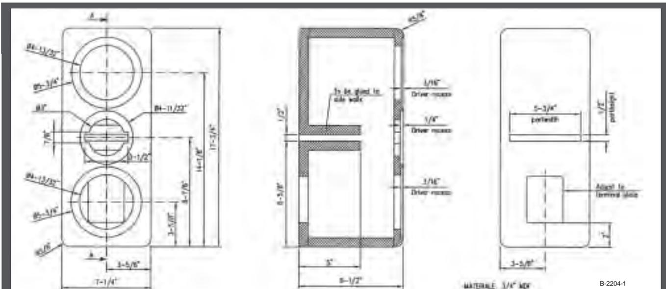
**FIGURE 1:** The SEAS cabinet drawing. The original was drawn in metric, which accounts for the tight diameters for the driver openings. The outer dimensions for cutting the dadoes are reasonable using the Jasper guide. The inner diameters are not so critical since they must only clear the cast frame of the drivers. Note that the sides of the cabinets fit inside the fronts, backs, tops, and bottoms.
