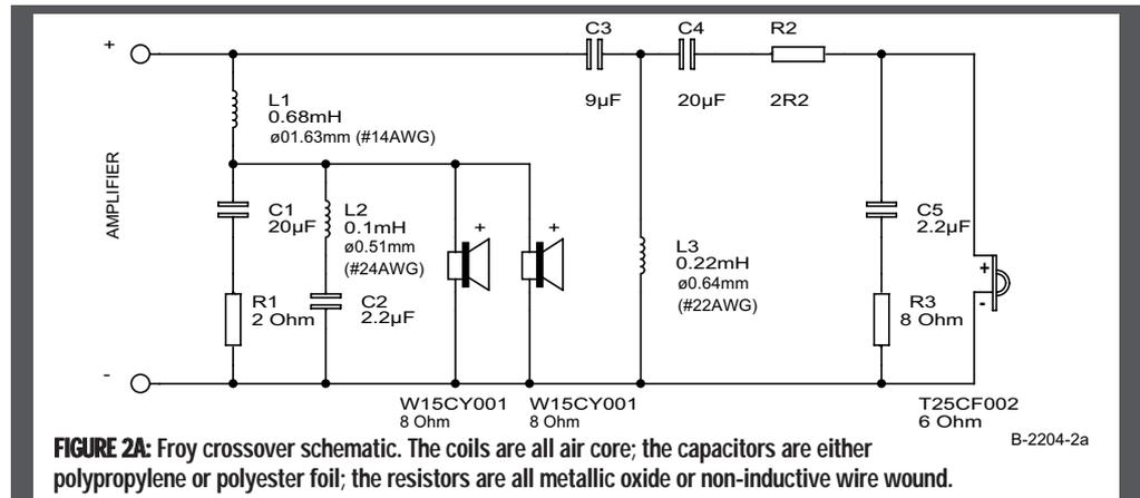
**FIGURE 2A:** Froy crossover schematic. The coils are all air core; the capacitors are either polypropylene or polyester foil; the resistors are all metallic oxide or non-inductive wire wound.
