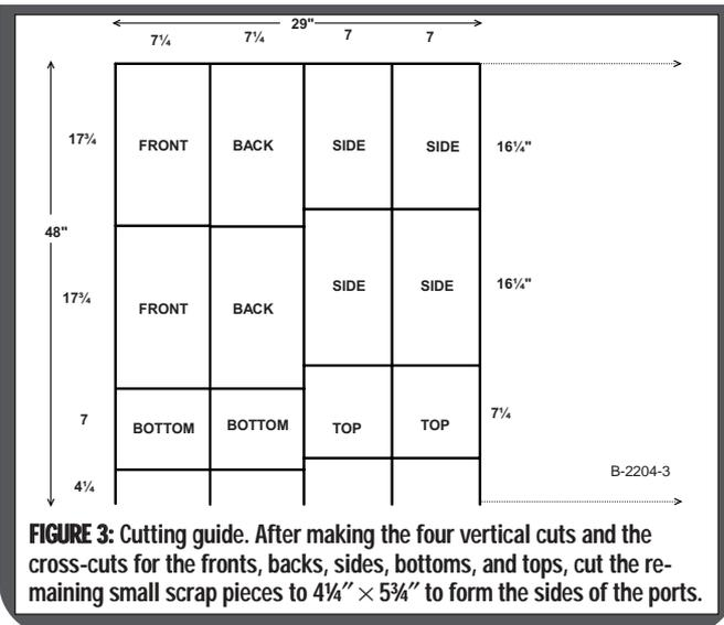
FIGURE 3: Cutting guide. After making the four vertical cuts and the cross-cuts for the fronts, backs, sides, bottoms, and tops, cut the remaining small scrap pieces to 4 1/4" x 5 3/4" to form the sides of the ports.
