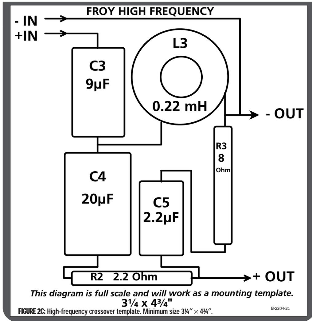
FIGURE 2C: High-frequency crossover template. Minimum size 3 1/4" x 4 3/4".
