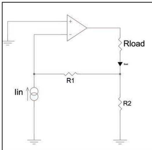
Figure 4: Transimpedance feedback gives rise to a transadmittance amplifier or a voltage-controlled current source (VCCS).
