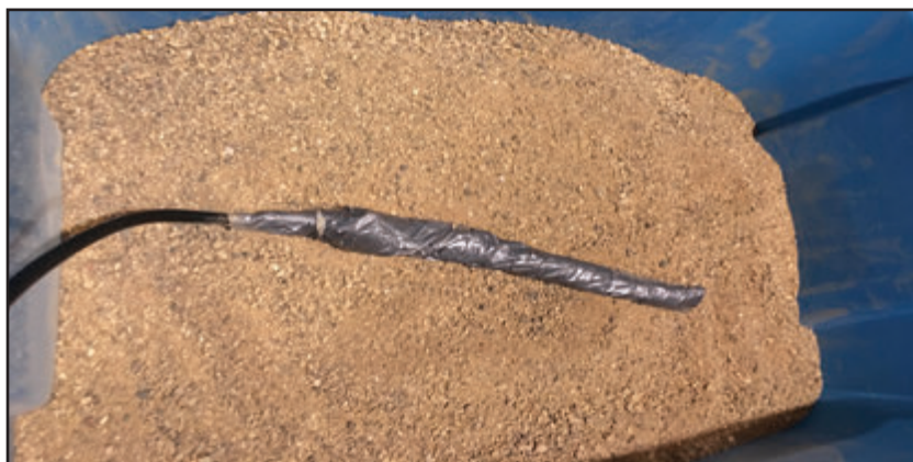
Photo 4: The BLANK method of noise floor measurement involves wrapping the microphone in plastic and duct tape to protect it, then burying in a mixture of sand and cat litter.
