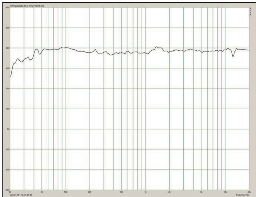
Figure 1: The Kii Three frequency response is flat between 30 Hz and 20 kHz.
