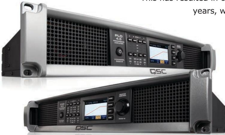
Photo 1: Housed in a 2U rack-mount configuration, CXD and PLD Series amplifiers feature new QSC proprietary Class-D power devices, which enable multichannel, high-performance power. Flexible Amplifier Summing Technology (FAST) provides better power allocation by actively distributing the total amplifier power across one, two, three, or all four outputs enabling amplifier channels to be combined for maximum current or voltage output.
