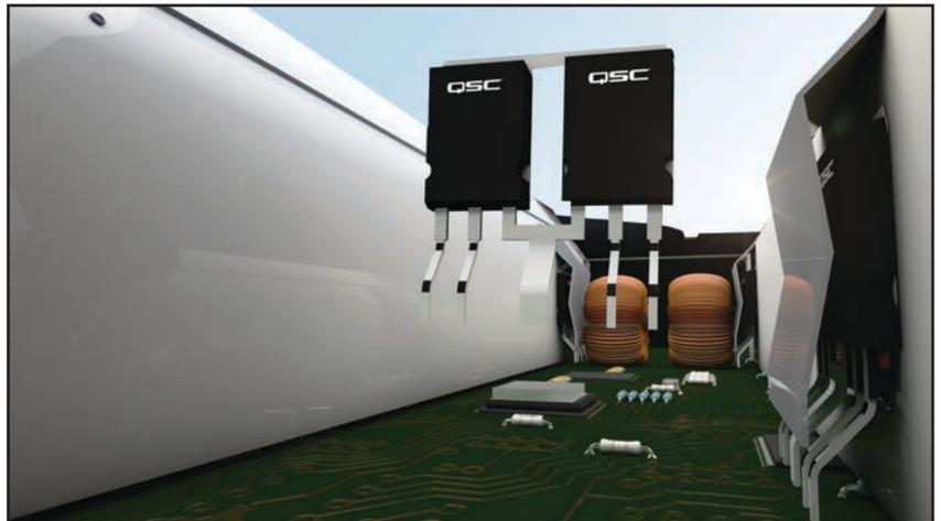
Photo 3: QSC's proprietary output MOSFET packaging contains two MOSFETs (presumably matched at the die phase) and steering circuitry.
