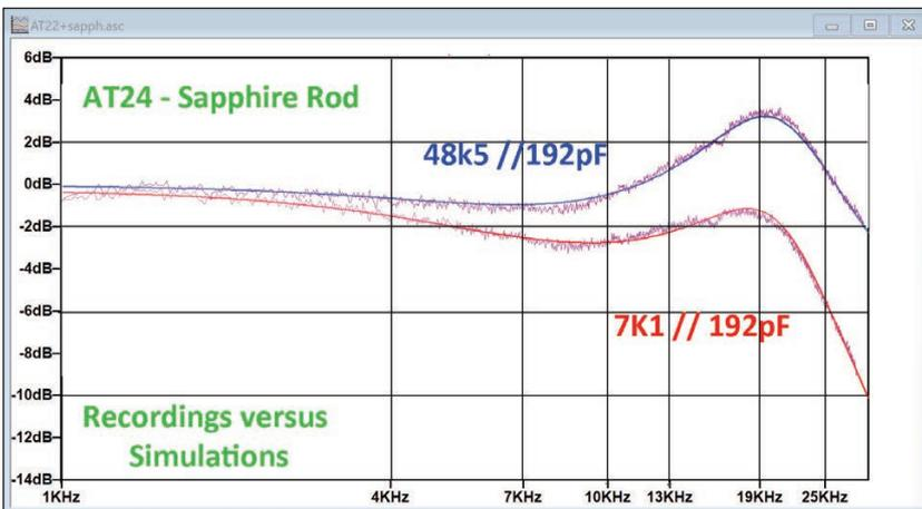
Figure 13: Recorded and simulated FR for two very different load situations.
