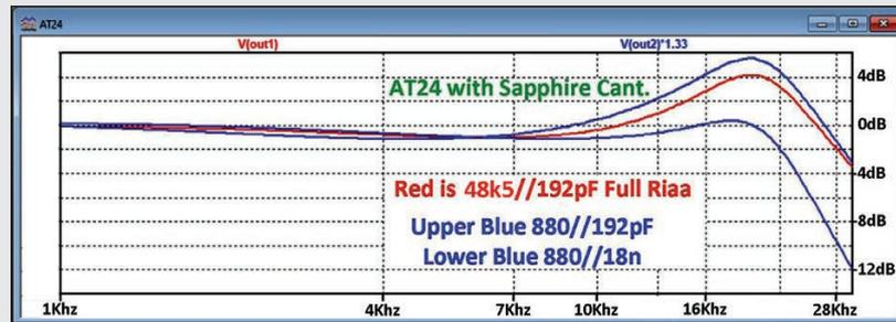
Figure 2: Loading the Cart with a 75µsec pole versus 48k5//192pF full RIAA.
