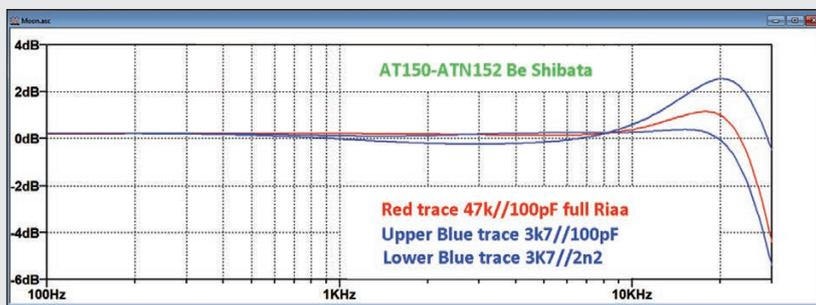
Figure 4: Loading the Cart with a 75µsec pole versus 47k//100pF full RIAA.
