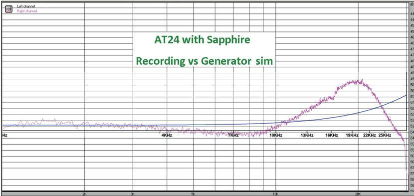
Figure 6: FR1 recorded with AT24 together with the FR2 simulated for its Generator, both terminated with 48.5kΩ (48k5) in parallel with 192pF.
