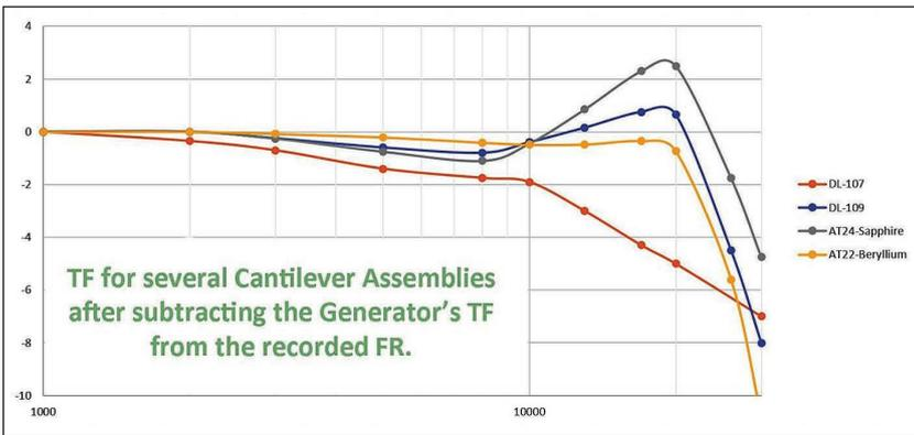
Figure 7: Transfer curves for four cantilever assemblies.
