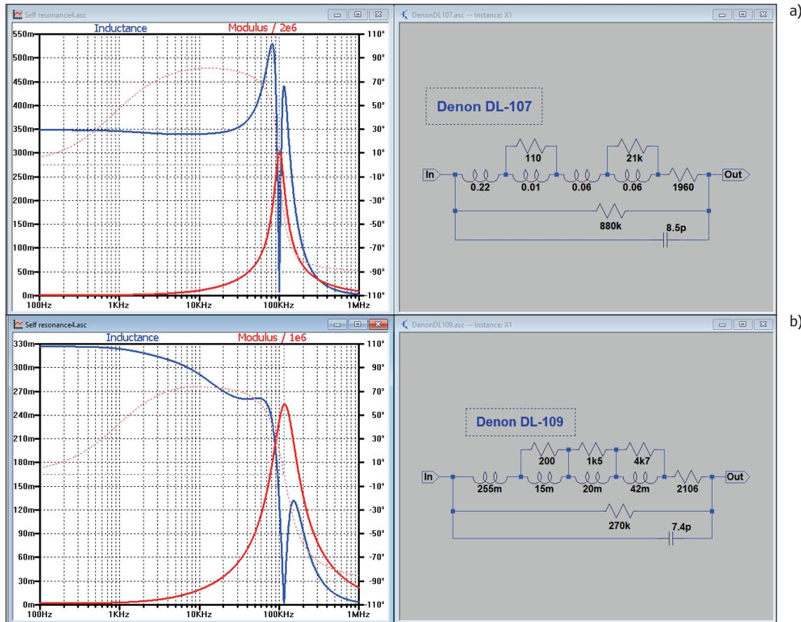
Figure 2: Circuit diagram for the Denon DL-107 (a) and the DL-109 (b).
