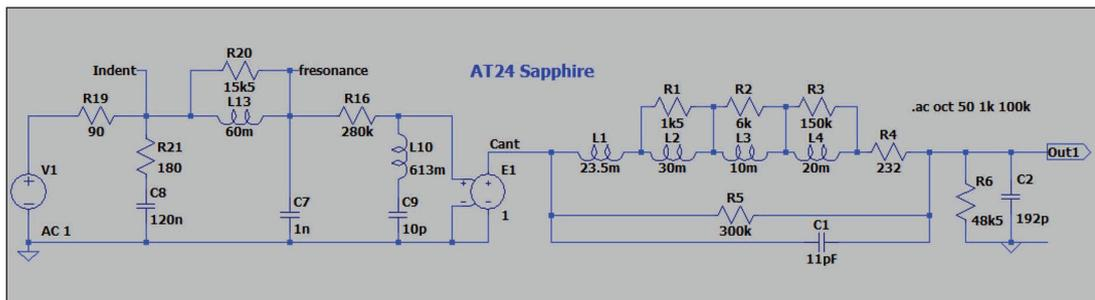
Figure 11: Circuit diagram for an AT24 with Sapphire cantilever and 0.24 mil elliptical tip.
