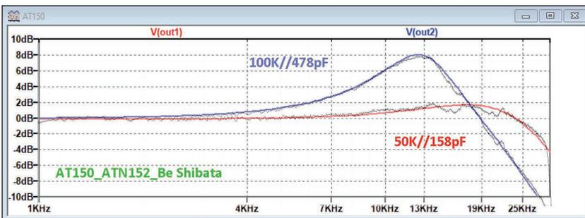
Figure 15: Recording versus simulation for a AT150 with ATN152 Cantilever.
