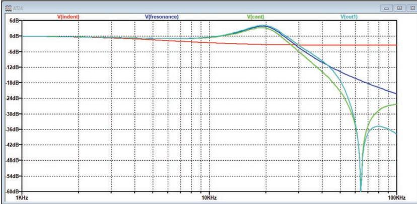
Figure 12: Frequency responses at various points from the AT24-Sapphire's circuit diagram.
