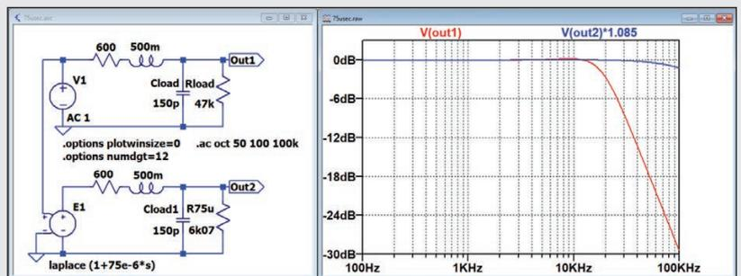
Figure 1: The effect of 75µsec damped loading on a simple Cart model.
