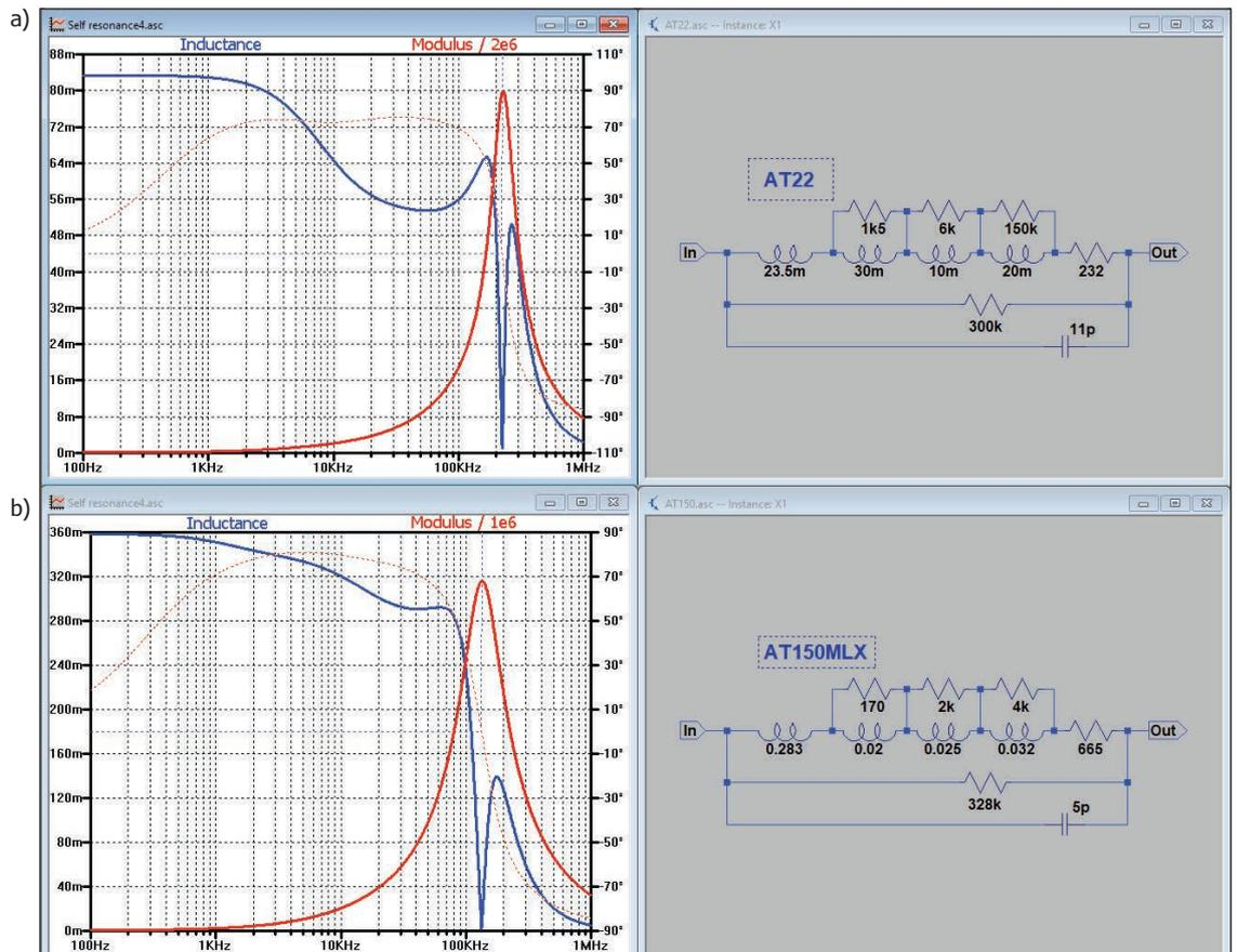
Figure 1: Circuit diagram for the Audio Technica AT22 (a) and AT150MLX (b).
