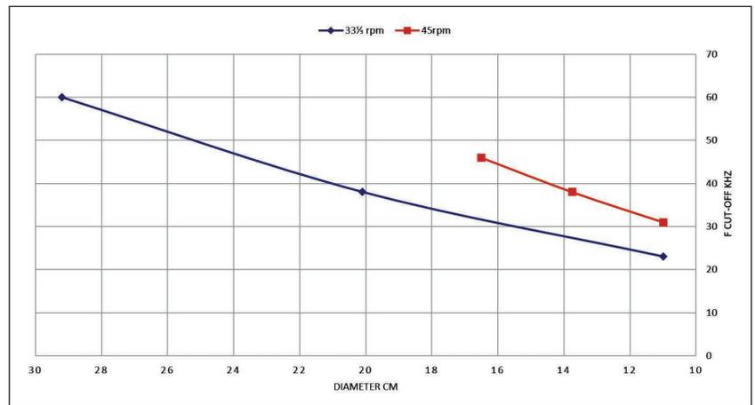
Figure 9: Cut-off frequency dependency on rpm and position for a 0.65 mil round tip.
