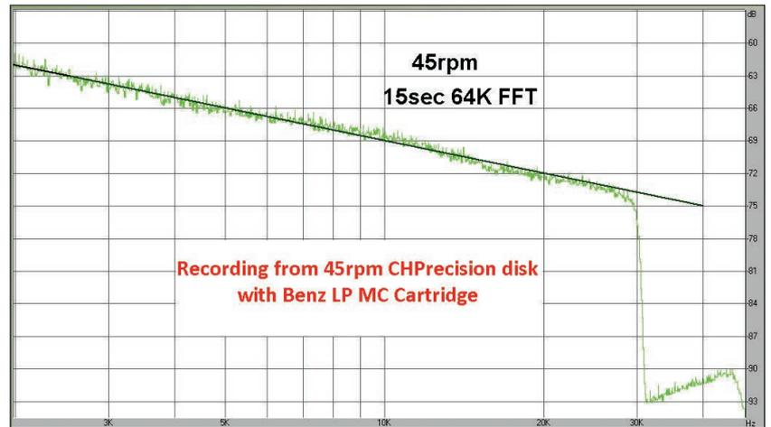
Figure 5: Checking the test signal on the CH Precision test disk.
