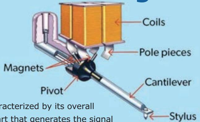
A moving magnet (MM) phono cartridge can be characterized by its overall transfer function. But the transfer function of the part that generates the signal through magnetic induction has its own transfer function, which can also be measured. By translating the latter into an equivalent electronic circuit, further insight and possibilities for optimization can be obtained. Hans Polak explains.
