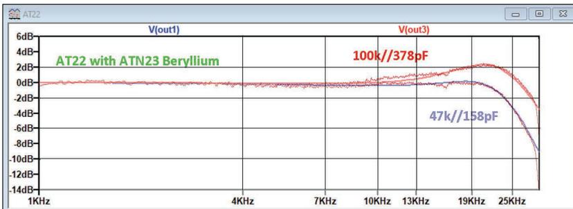
Figure 14: Recording versus simulation for a AT22 with ATN23 Cantilever.
