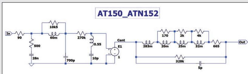
Figure 3: Equivalent diagram for the AT150 with 5µm ATN152 Beryllium Shibata tip.
