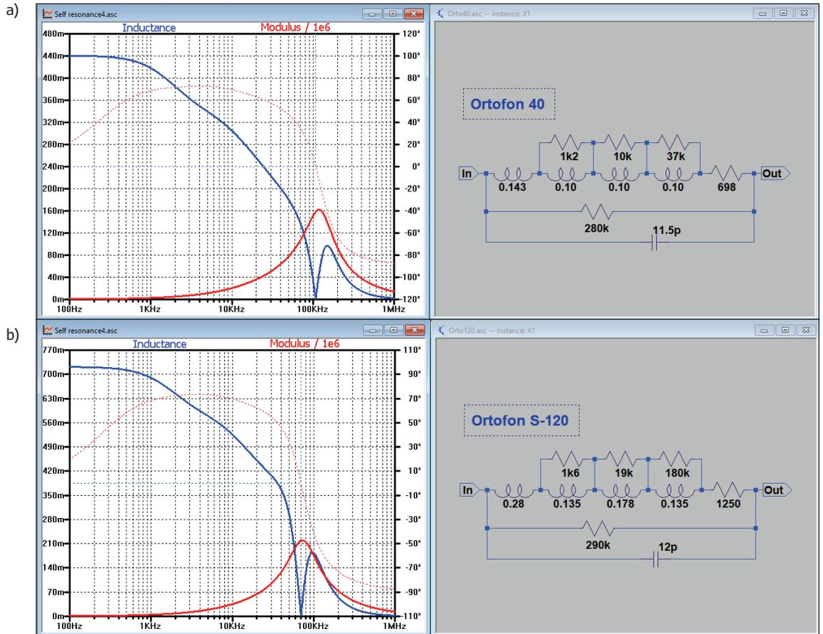
Figure 3: Circuit diagram for the Ortofon 40 (a) and the Ortofon S-120 (b).
