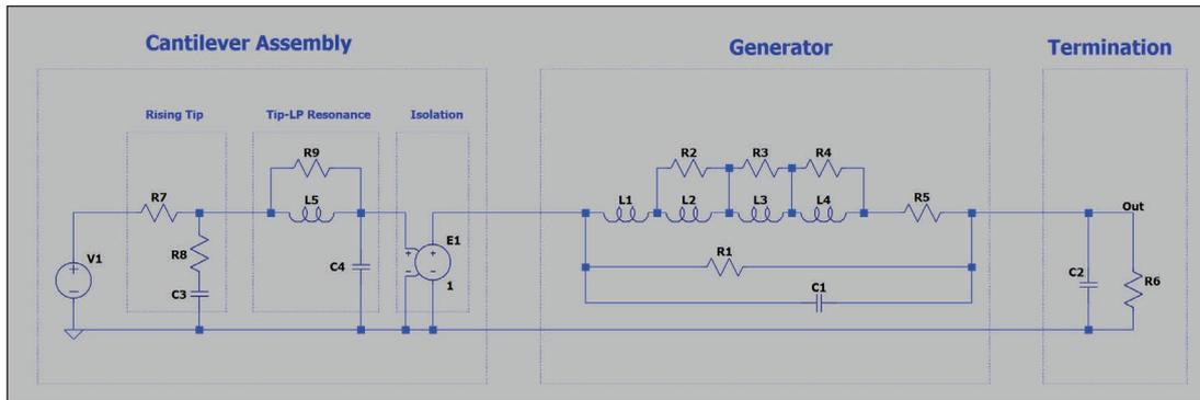
Figure 10: Generic model for cartridge plus termination.
