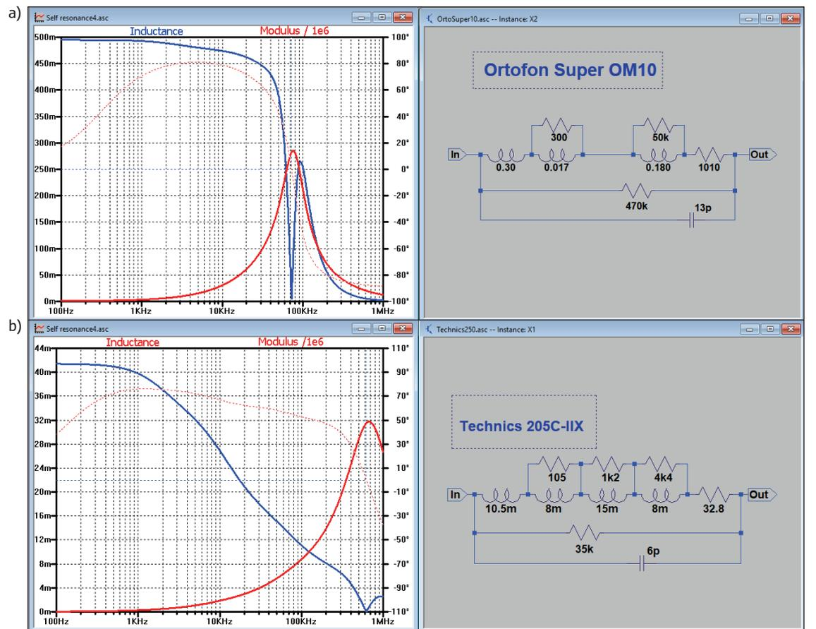
Figure 4: Circuit diagram for the Ortofon Super OM10 (a) and the Technics 205C-IIX (b).
