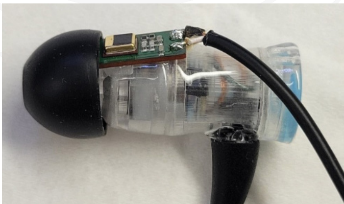
Figure 3. Knowles K-1 hybrid earphone, with MEMS mic attached to monitor the response.
