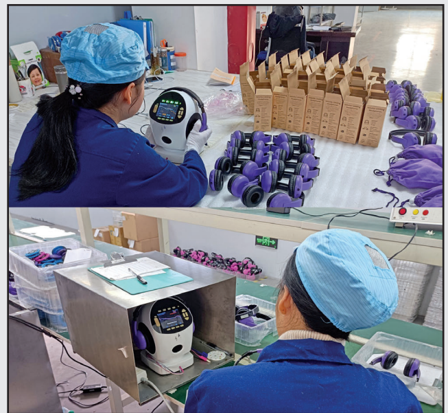
Production line testing and quality control of headphones from ONANOFF
