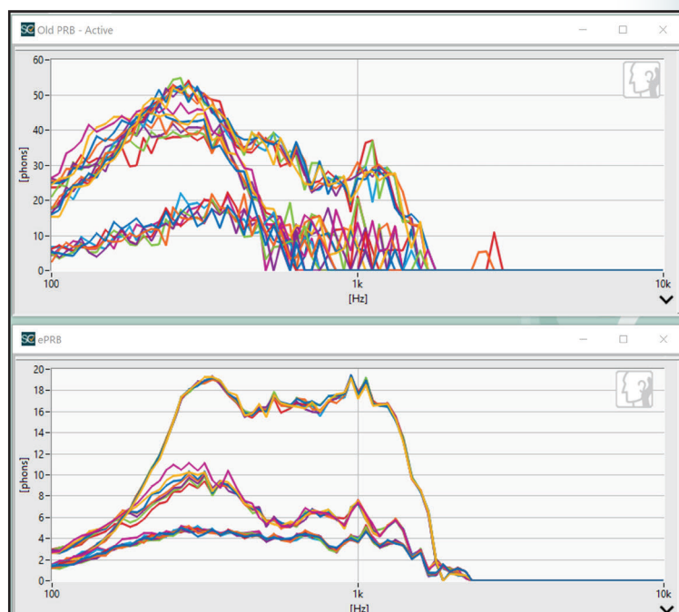
Comparison of Listen's new Enhanced Perceptual Rub & Buzz (ePRB) Algorithm (lower) with the original Perceptual Rub & Buzz (PRB) Algorithm (top)
