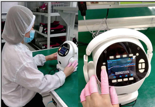
The ZUMI HPA85 headphone test system in use in a factory in China
