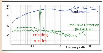
Figure 1: Frequency response of SPL fundamental component and impulsive distortion measured with a stepped sine stimulus (dashed line) and continuous log chirp with speed profile (solid line) using the same total stimulus length of 200 ms.
