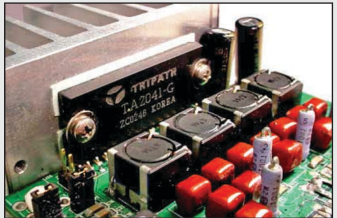
Photo 2: A Tripath TA2041 four-channel amplifier was rated at a maximum output of 280 W (70 W per channel).
