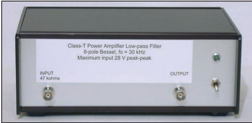
Photo 3: A front view of the active low-pass filter used in the Class-T amplifier testing to remove the output high frequency switching noise is shown. This filter was not used for the transient response test.
