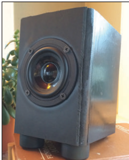
Photo 1: DSP makes it possible for a 3" full-range driver (Fountek FR89EX) and 5" passive radiator (rear mounted) to achieve 55 Hz to 20 kHz in a tiny 1-ltr box with surprisingly high output.
