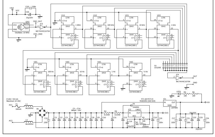
Figure 6: The electronic diagram of the Reference Oscillator
