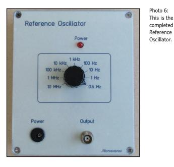
I used an aluminum enclosure to house the PCB and the connectors. Using the "Front Panel Designer" program, I also designed a front panel for the unit. The result was a more professional-looking device that was also easy to operate. I attached the PCB to the front panel using as support the switch, which I placed at the center of the PCB. A BNC connector is used for the output of the oscillator. Photo 6 shows a view of the completed reference oscillator.
