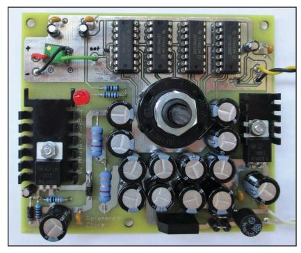
Photo 5: This is a top view of the Reference Oscillator's completed PCB.
