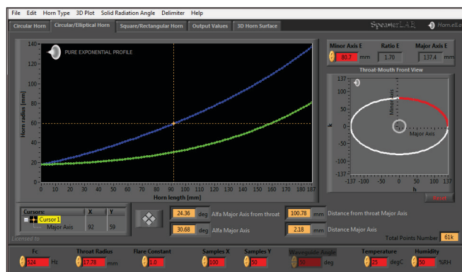
Figure 18: Elliptical mouth horn's arrangement. MR = 1.7
