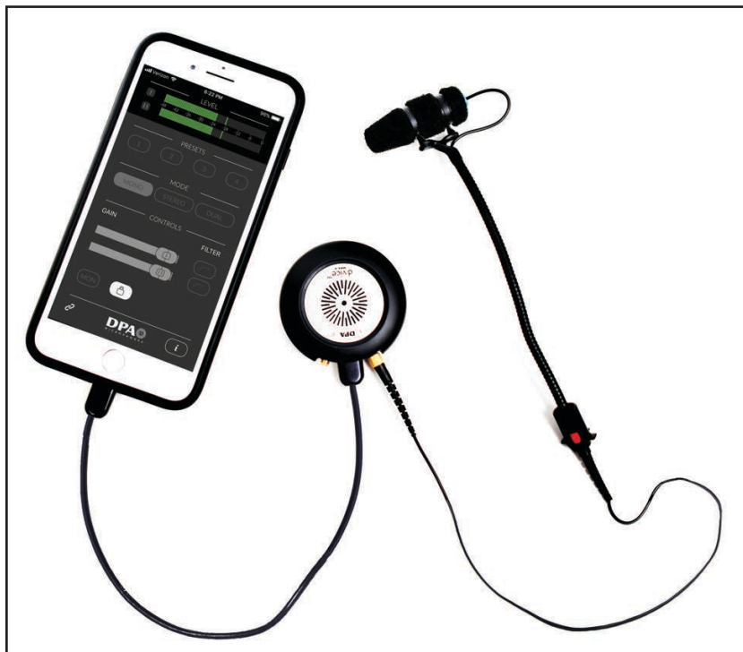
Photo 6: Connecting microphones to an iPhone through the MMA-A is simple and straightforward, creating a very portable and high quality recording system. (Photo courtesy of Cynthia Wenslow)
