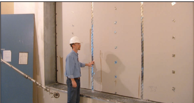
Photo 4: The author oversees one of the ASTM E-90 TL tests in the source side reverberation chamber. These are actual wall constructions filling an 8' wide by 12' tall chamber opening between the source and receive reverberation chambers.
