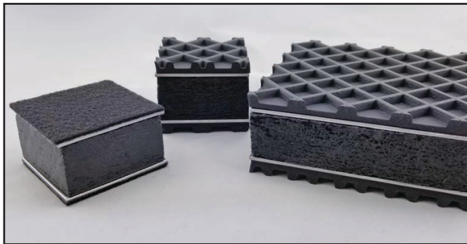
Photo 5: Equipment Vibration Protectors (EVPs) are available in 2" and 4" squares by approximately 1" tall, with felt and rubber finishes, and in three standard densities to handle equipment loads from 3 lbs to more than 300 lbs.
