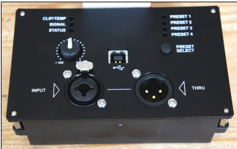
Photo 5: The assembled DSP Lite module with front plate
