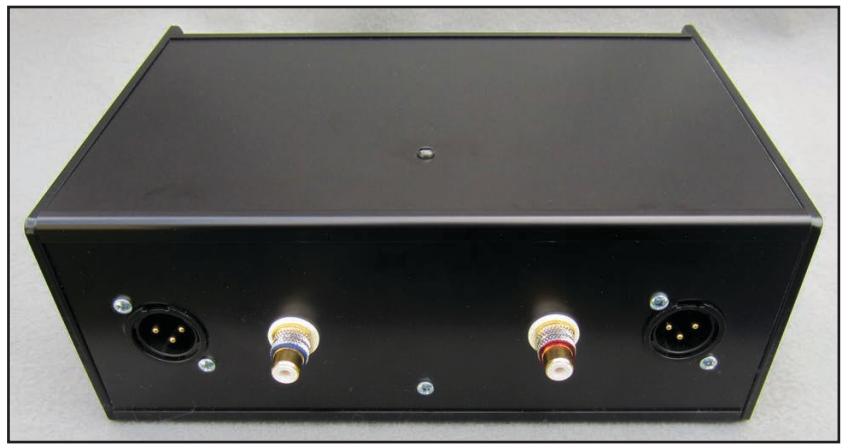
Photo 3: This is the rear view of the enclosure, showing the unbalanced RCA inputs and the balanced XLR outputs.
