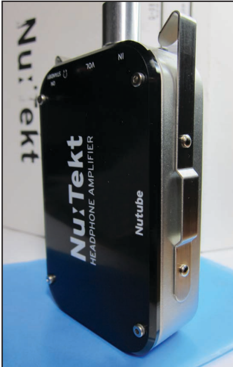
Photo 5: This is how the Nu:Tekt amp should look when fully assembled.
