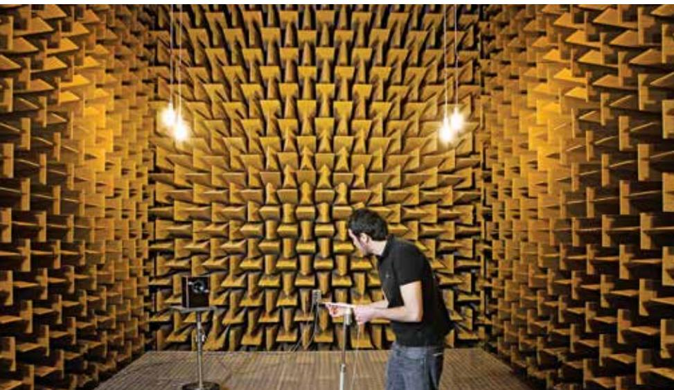
**01** An anechoic chamber consists of a shell of concrete and Leca that rests on coil springs to dampen noise from vibration in the ground. The chamber is lined on the inside with meter-long sound absorbing wedges of damping material. The chamber is used for all kinds of free field measurements.
