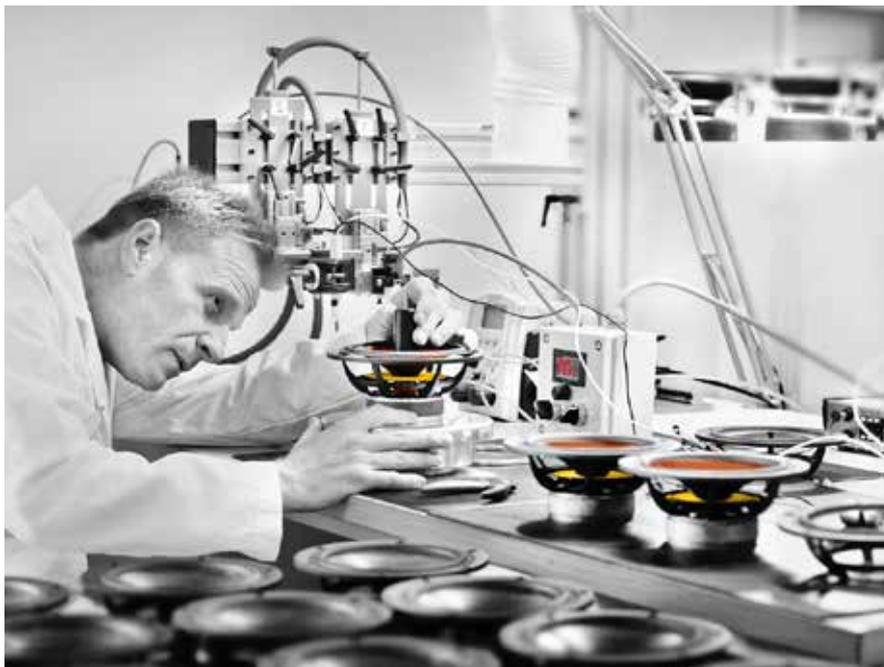
*Loudspeaker drive manufacturing in-house was from the start a close cooperation between R&D and production engineers.*
