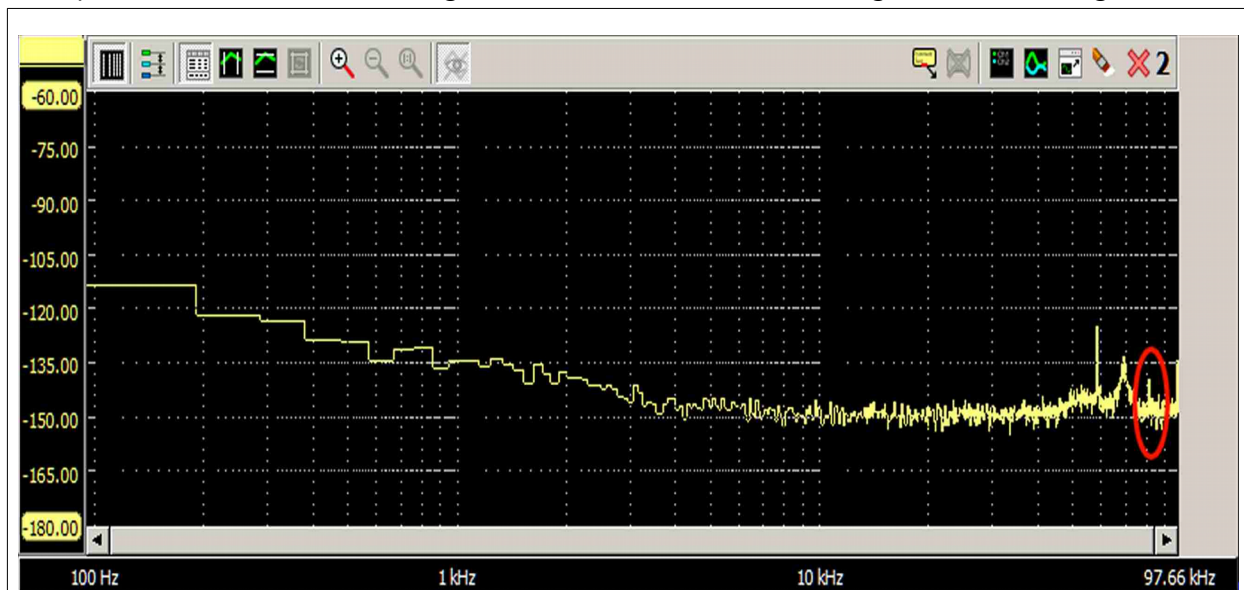
Figure 5 HS3 ground noise, USB with phone
