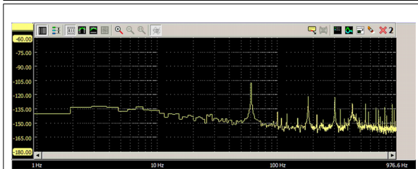
Figure 11 WaveTek source at 100Hz, LT3045
