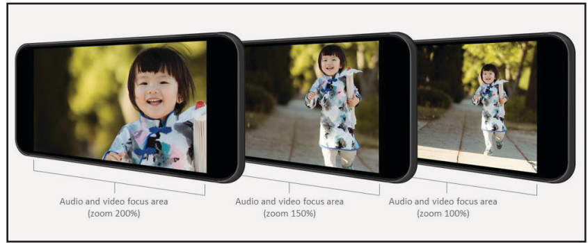
Figure 3. This is a UI demonstration of how Audio Zoom automatically and dynamically adjusts audio focus to the area of the zoomed video.
