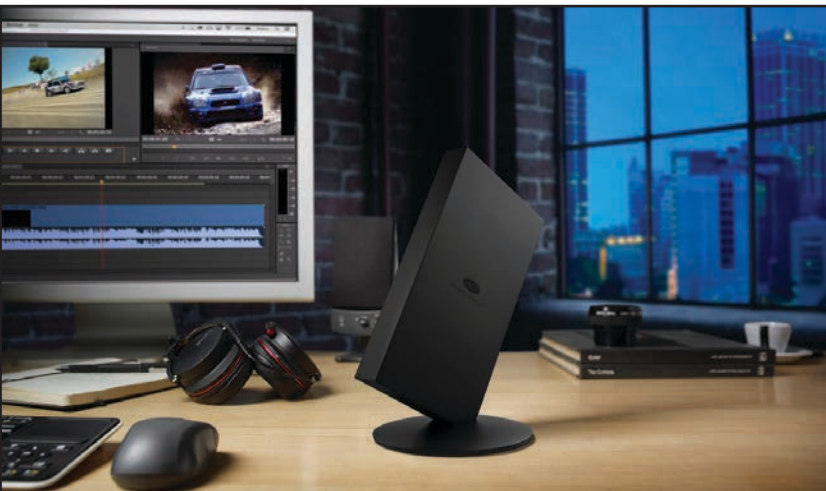
The new LaCie Bolt3 external drive (2x M.2 PCIe SSDs) uses dual Thunderbolt 3 to achieve 2,800 MB/second read and 2,200 MB/second write speeds.
