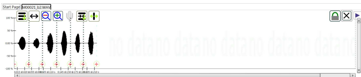
The same signal after it has been compressed. Most of the silence between the pulses is now hidden.
