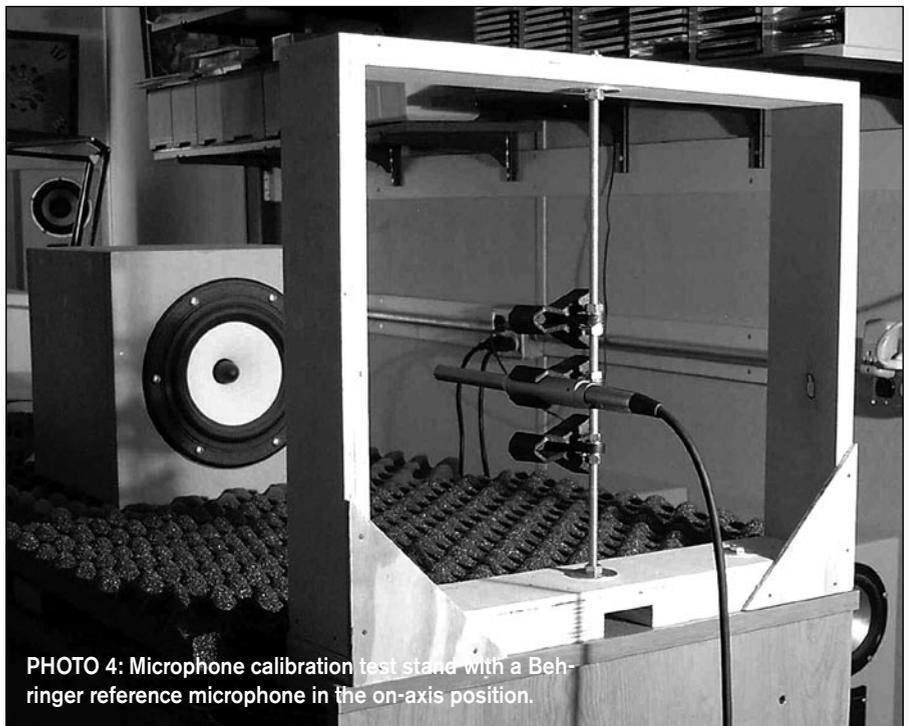
**PHOTO 4:** Microphone calibration test stand with a Behringer reference microphone in the on-axis position.
