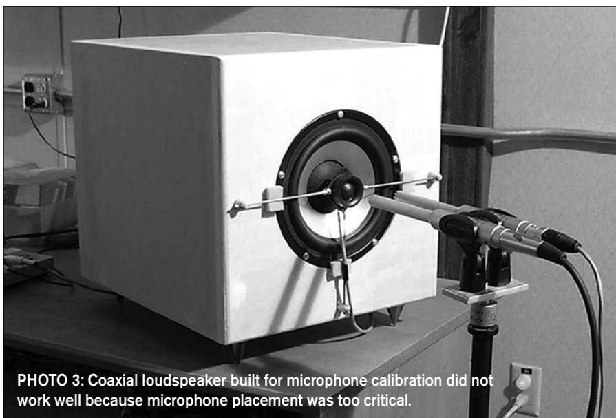
1. Reference microphone, Behringer ECM-8000<sup>6</sup>. (It would be helpful to buy three, as I will explain later.) You will notice that the microphone spec sheet indicates +15 to +48V of phantom power is needed, which is true. But at 15V the sensitivity has decreased and the decrease isn't specified. I have measured it at about -2.5dB, but it varies from microphone to microphone.
