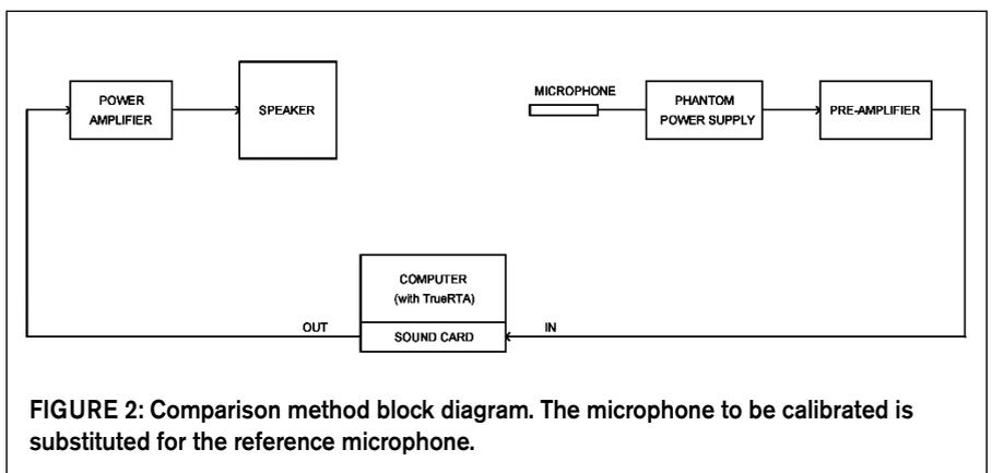
**FIGURE 2:** Comparison method block diagram. The microphone to be calibrated is substituted for the reference microphone.
