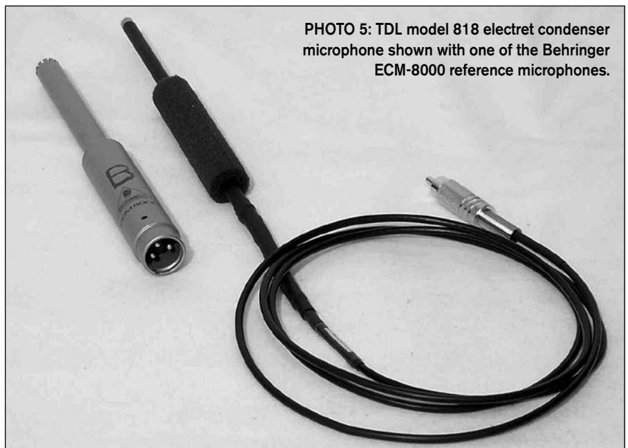
**PHOTO 5:** TDL model 818 electret condenser microphone shown with one of the Behringer ECM-8000 reference microphones.
