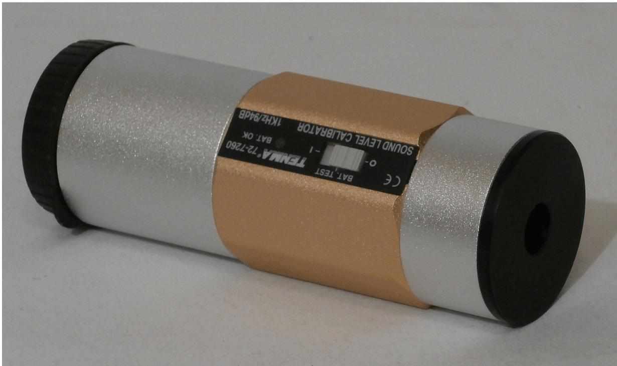
This calibrator generates a low-distortion 1,000 Hz sine wave at 94 dB SPL. The microphone to be calibrated is inserted into the ½" diameter well in the "business end" and the battery-powered unit is turned on. Both the above microphones have ½" barrels so they can be easily measured. But an adapter must be used for the smaller diameter of the WM-61A.
