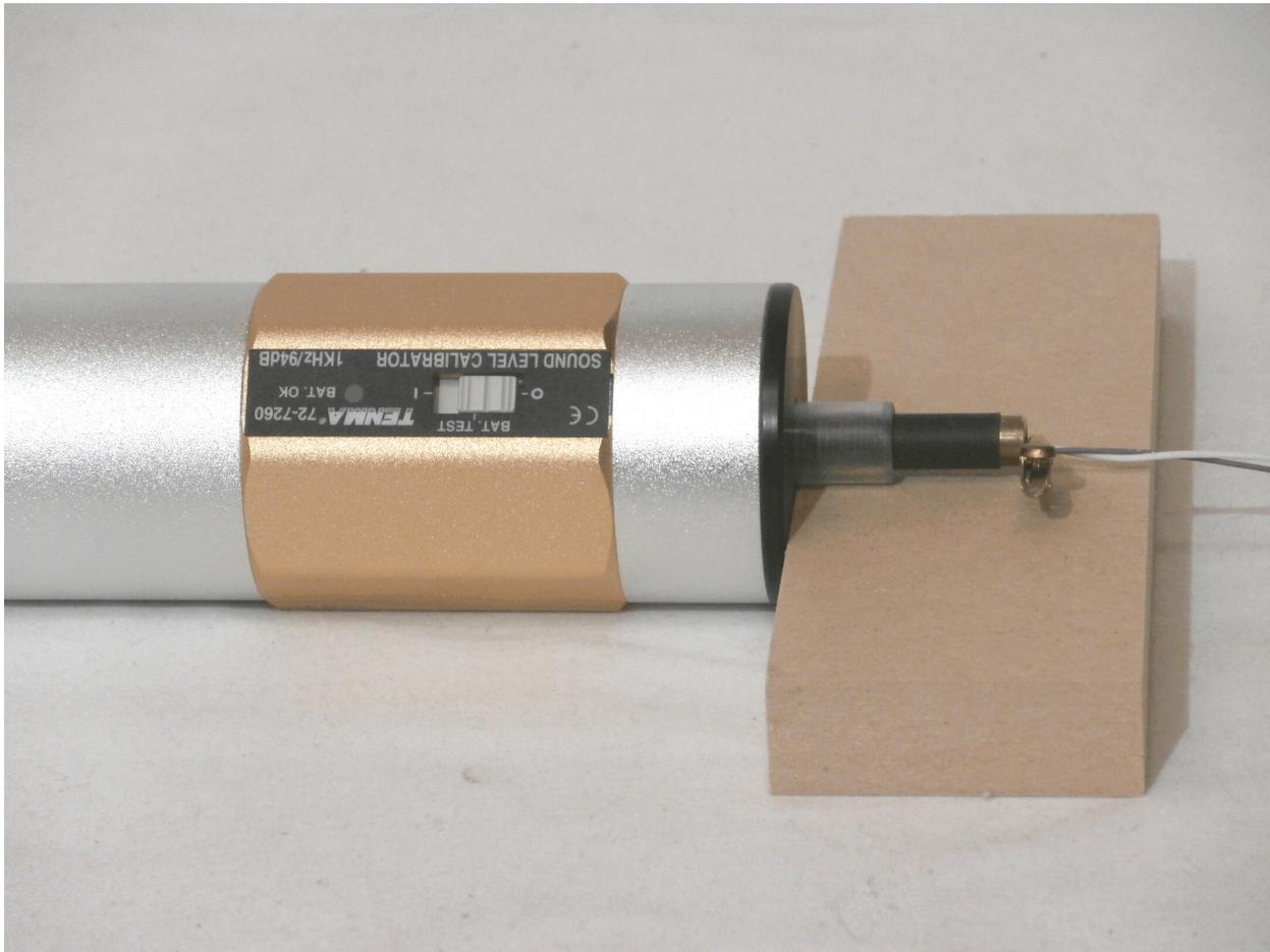
The WM-61A needs a minimum 2 volts DC with a maximum of 10 volts. A microphone preamp with 5 volts is ideal. The preamp SHOULD have a switch to set the gain because it's all too easy to slightly move a pot's setting. For cartridge matching, the absolute gain is not important but it MUST remain constant for all the cartridges Connect an AC voltmeter (I prefer a digital meter) to the preamp's output and start measuring!
