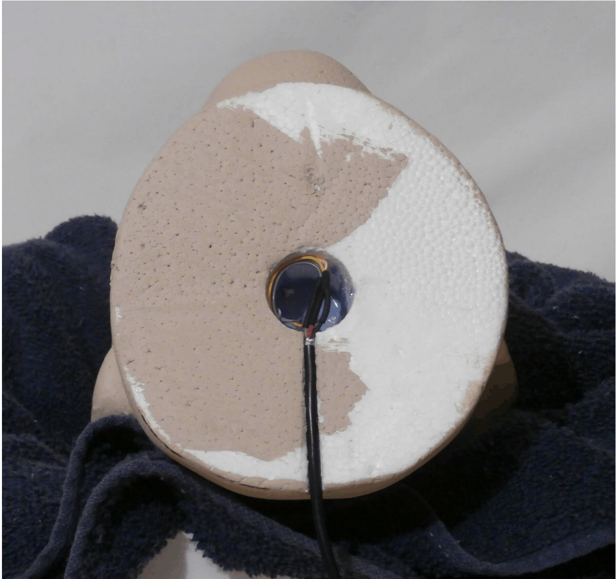
Photo 7 – When the wires have been spliced, they are tucked into the center hole and the microphone cable is laid in its groove.
