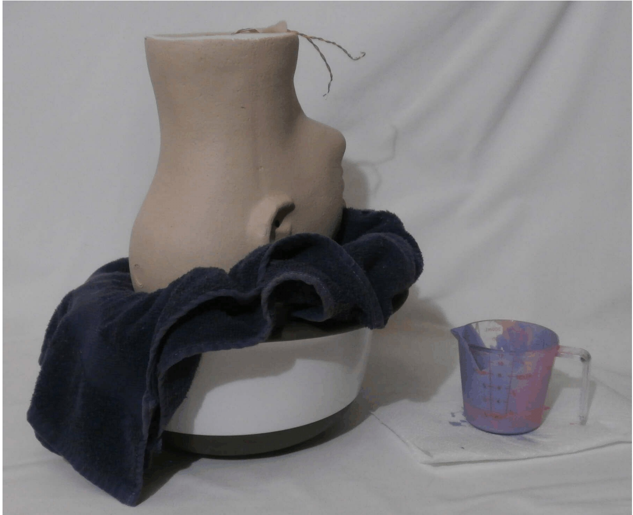
Photo 4 – With the head model upside down, slowly pour the liquid rubber mixture into the center hole until the level is about an inch from the top. This leaves space for the splices connecting the microphone wires to the shielded microphone cable. The rubber takes about 6 hours to cure.
