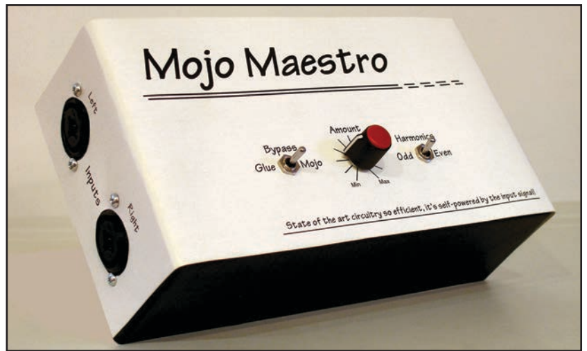
Photo 1: I used Microsoft Visio to design the connector layout, front panel holes, and label the plastic project case.
