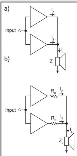
Figure 2: Parallel two amplifiers to make a single amplifier with higher output current capability. The basic paralleling topography—ideally  $I_A = I_B$ —enables all current to be equally shared and delivered to the load (a). Use ballast resistors to equalize current draw from each amplifier in the parallel pair (b).
