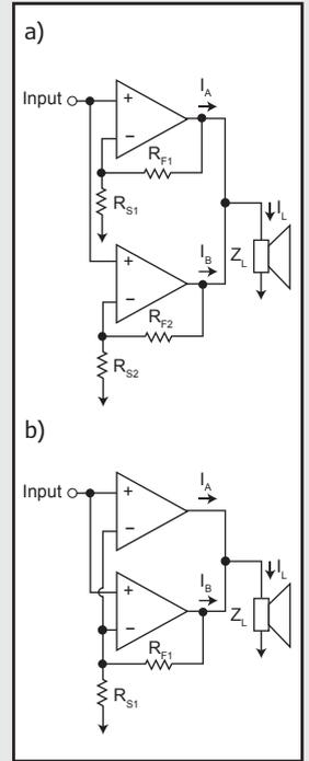
Figure 3: Feedback systems can be used for paralleled amplifiers. Conventional approach—tolerances in the feedback components mean that one amp drives current into the other (a). QSC’s single feedback system is automatically implemented when channels are paralleled (b).
