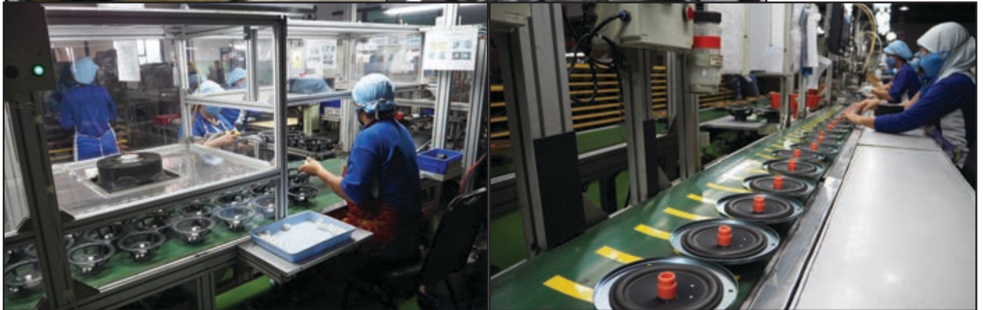
Speaker assembly lines. Sinar Baja Electric has surpassed the TS 16949 requirements for automotive standards and for ISO 9001 quality certifications.
