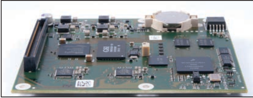
ALC NetworkX's COMi.MX board is a complete SoM solution for quick and easy OEM RAVENNA/AES67 integration, complemented by a C/C++ software framework and reference design including a full source code package.
