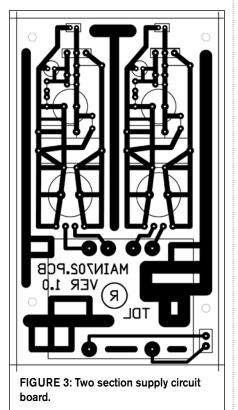
supplies. The circuit board layouts (single-sided) are shown in **Figs. 2** and **3**. (You can download the layout files from the TDL<sup>®</sup> website.<sup>1</sup>) I named this supply a Model 701 (just to keep track of circuit boards and parts), but it is not a product, and I have built only the one prototype. Hence, the front panel has no labels.
