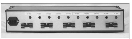
PHOTO 3: Multiple wall-wart power supply rear panel. During continuous operation, the panel is only slightly warm to the touch.
