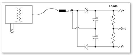
FIGURE 1: Wall wart used with voltage doubler. In this and subsequent drawings, resistors hanging on the DC outputs of the supplies represent their loads. Note that the ground is produced at the junction of the two legs of the load, not within the supply itself.
