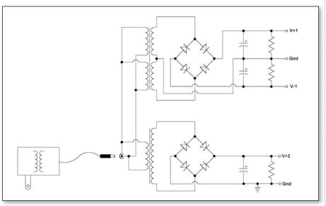
FIGURE 6: Using two additional transformers to derive three DC voltages from a single wall wart.
