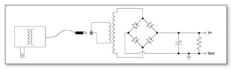
FIGURE 5: Using a second transformer to step up the voltage of a wall wart.
