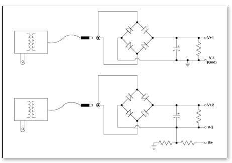
FIGURE 4: Two filament supplies for tubed circuits; the first is referenced to ground, the second to a voltage divider from the plate supply, scaled to hoist the filament about 80V above ground.
