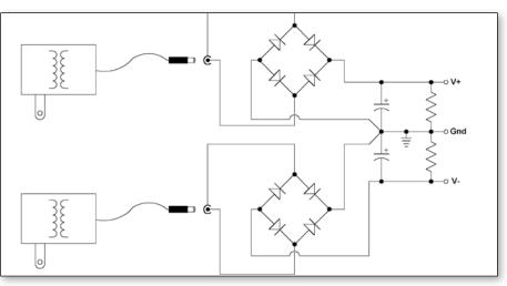
FIGURE 3: Two wall warts with separate diode bridges.
