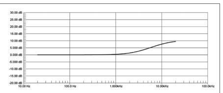
FIGURE 1: The Red Book pre-emphasis curve specifies time constants of  $50\mu$ S and 15 $\mu$ s. The +3dB point for the high-frequency boost is 3183Hz, shelving at 10610Hz. Maximum boost is +9.49dB at 20kHz.
