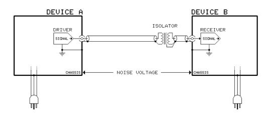
Transformers make excellent ground isolators. They transfer signal voltage from winding to winding without any electrical connection between them. This opens the path of the noise current that would otherwise flow between devices.
