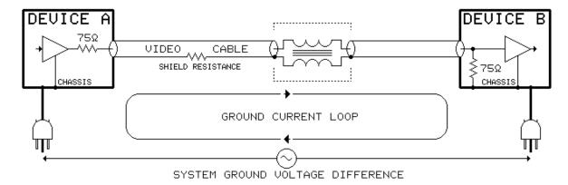
Referring to the schematic, note that the video *signal* current flows from device A to device B through the upper winding and returns through the bottom winding. Because the two windings
