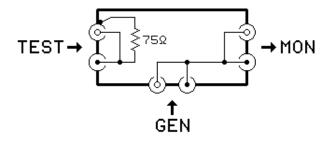
By temporarily placing the dummy and generator at strategic locations in the system, precise information about the nature of the problem is revealed. The cable between the dummy and Box B must be as short as possible and much shorter than the cable under test. Always start at the input to the display and WORK BACKWARDS toward the signal sources.
