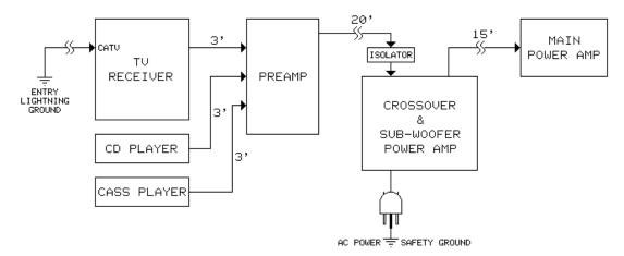
Another **safe** solution is to break the loop by installing a ground isolator in the CATV signal path at the TV as shown. CATV isolators should generally be installed where the cable first connects to the audio or video system, such as at a VCR or TV receiver input.
