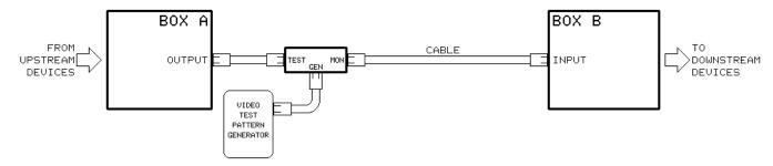
Disturbance gone? **No** — ground current is being coupled by the common-impedance of the cable shield. Install a suitable ground isolator device.
