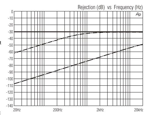
60 Hz and about 65 dB at 3 kHz. For the best possible noise rejection, don't use a 2-conductor cable from the unbalanced output to the isolator input. Instead, use a balanced (XLR connector) input and the 3-conductor cable wired as in the alternate hookup. These tests were done using a 600  $\Omega$  unbalanced output and the same 40 k $\Omega$  balanced input described in section **3.5**.
