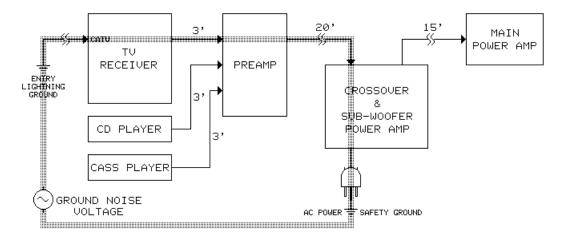
loop between the TV and the sub-woofer. Thus, common-impedance coupling will introduce noise in both *audio* cables in the path, generally in proportion to their lengths. This system would exhibit a loud hum regardless of preamp control settings because of coupling in the 20-foot cable.
