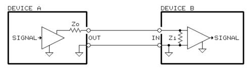
depending **only** on the **impedances** (to ground) of the line's two conductors. As shown above, in an **unbalanced** interface, one conductor is grounded (zero-impedance) and the other has some higher impedance.
