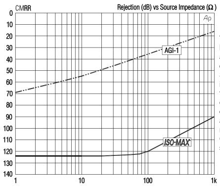
The plots at left compare the 60 Hz hum rejection performance of another typical active interface device, the now discontinued Sonance AGI-1 "audio ground isolator," to that of an inputtransformer based isolator. Over the consumer output impedance range of 200  $\Omega$  to 1 k $\Omega$ , the *active* isolator achieves only 15 to 30 dB of rejection while the ISO-MAX® CI-2RR isolator improves that by some 80 dB!
