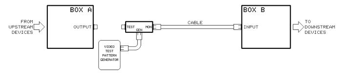
Disturbance gone? **No** — the disturbance is being induced in the cable itself. This is most often caused by a strong ac magnetic field near the cable. Re-route the cable to avoid the strong field. Sources of such fields include high-current power wiring, power transformers, and CRT displays. Electric field coupling is also possible, but *extremely* rare in video systems unless the shield itself is broken or disconnected.
