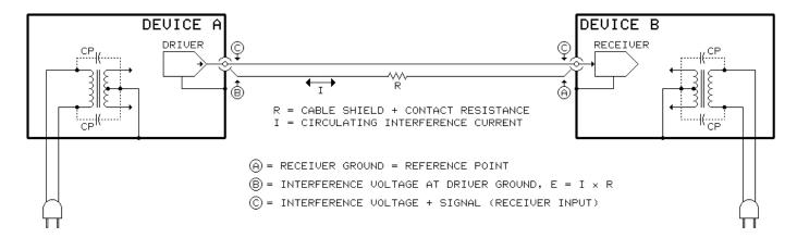
Consider a 25-foot interconnect cable with foil shield and a #26 AWG drain wire. From standard wire tables (or actual measurement) its shield resistance is found to be 1.0  $\Omega$ . The resistance of the inner conductor is insignificant and is not discussed here. If the leakage current is 316  $\mu$ A, the
