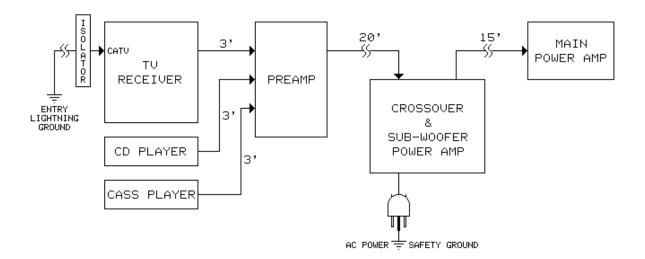
Since most consumer equipment uses 2-prong ac plugs (ungrounded), installing an isolator may leave some devices "floating." This can allow the voltage between the input and output ports of an isolator to approach 120 volts ac.
