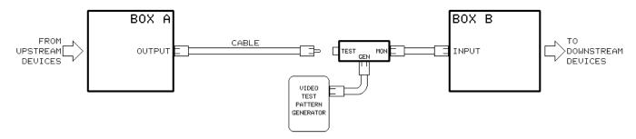
Disturbance gone? **No** — the problem is either with Box B or further downstream. Reconnect the cable and perform this test on the next downstream interface. **Yes** — go to next step.
