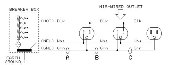
grounded equipment. This error *cannot* be found with simple outlet testers, but measuring current at points A, B, and C with a clamp-on ammeter will clearly reveal it. [30]
