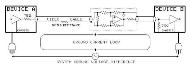
differential amplifier devices require a "trim" adjustment to achieve maximum common-mode rejection. This might be a disadvantage in portable systems where cables are frequently changed or re-routed. Although differential amplifiers require power and contain active circuitry, features such as multiple outputs and adjustable gain can be useful.
