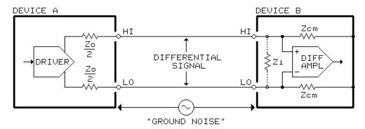
Theoretically, it can reject any interference, whether due to ground voltage differences, magnetic fields, or electric fields, as long as it produces *identical* voltages each of the signal lines and the resulting peak voltages don't exceed receiver
