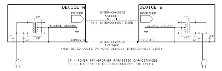
In UL-approved ungrounded (i.e., 2-prong ac power plug) devices, this current is limited to 0.75 mA. Such equipment incorporates a number of protective mechanisms so that it remains
