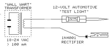
current of about 50 mA to flow through the potentially troublesome shield connections in the device under test. In *properly* designed equipment, this causes no additional noise at the equipment output. The diode is used to create easily audible harmonics of 60 Hz and the lamp is useful to show that a good connection has been made and current is indeed flowing.
