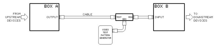
Disturbance gone? **No** — the problem may be due to common-impedance coupling inside Box B or a device farther downstream. If the input is differential (i.e., shield not directly grounded), the problem may be due to exceeding its common-mode voltage limits. If the problem is not in Box B, reconnect the cable and begin the test procedure on the next downstream interface. **Yes** — go to next step.
