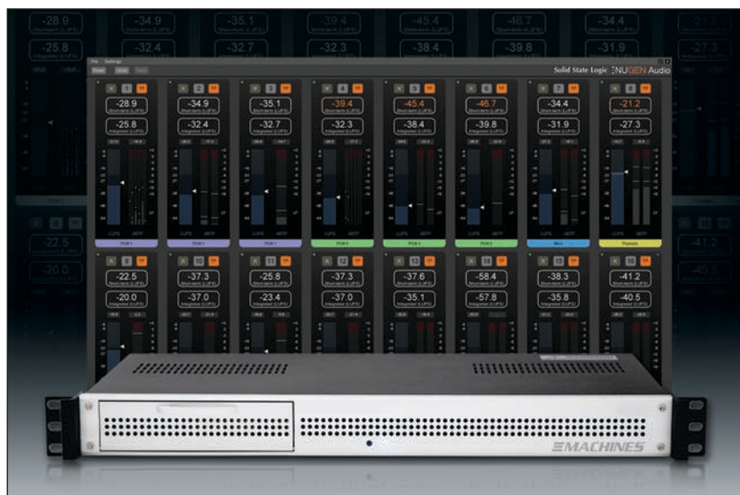
Photo 8: Solid State Logic introduced the LMS-16, a new multichannel Loudness and True Peak metering system developed in cooperation with Nugen Audio. The Nugen MultiMonitor was also presented as a stand-alone software product.
