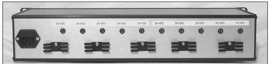
**PHOTO 3:** Multiple wall-wart power supply rear panel. During continuous operation, the panel is only slightly warm to the touch.
