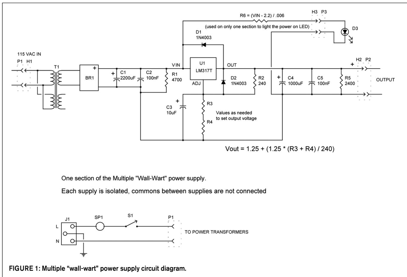
FIGURE 1: Multiple “wall-wart” power supply circuit diagram.
