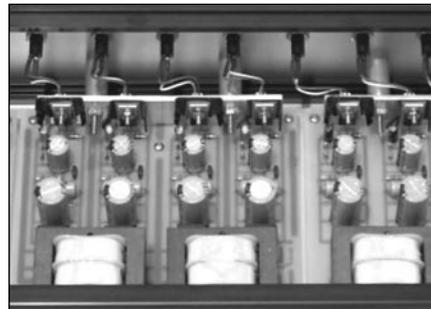
**PHOTO 2:** Multiple wall-wart power supply inside view. After mounting the circuit boards, measure the distance from the aluminum heatsink bar to the rear panel and cut the 1/2" diameter aluminum rod to this length.
